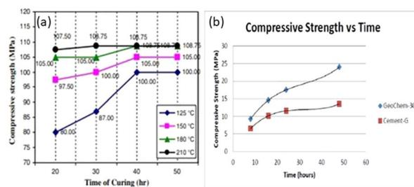
Fig. 41 (a) Compressive strength development of a geopolymer after curing for 7 days at different temperatures. (b) Compressive strength development of a geopolymer with time.<sup>144</sup>
