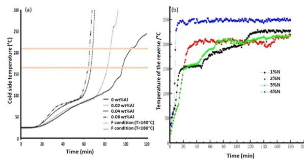
Fig. 24 (a) Fire testing of 4 different mixtures of metakaolin geopolymer. (b) Fire resistance test of metakaolin geopolymer activated with Na<sub>2</sub>O<sub>2</sub>; N shows percentage of Na<sub>2</sub>O<sub>2</sub>.<sup>35,124</sup>
