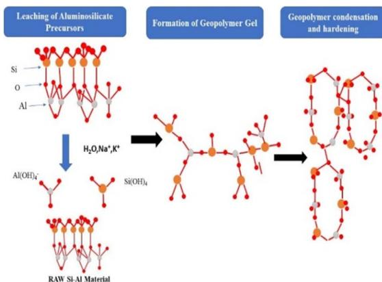
Fig. 15 Graphical model of geopolymerization process (orange circle represents Si, red circles represent "O" and grey circles represents "Al").<sup>92</sup>
