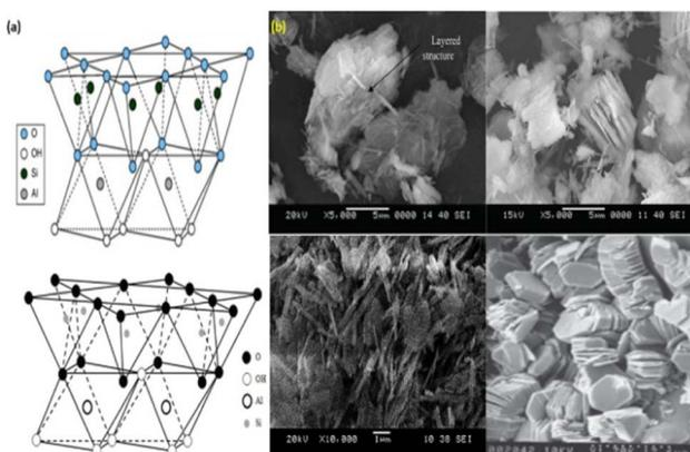
Fig. 3 (a) Kaolinite structure and (b) microstructure of kaolinite.<sup>4–7</sup>
