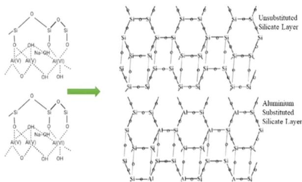
Fig. 12 Schematic showing the unsubstituted silicate layer and substituted aluminium silicate layer after interaction of metakaolin with NaOH solution.<sup>6,86</sup>
