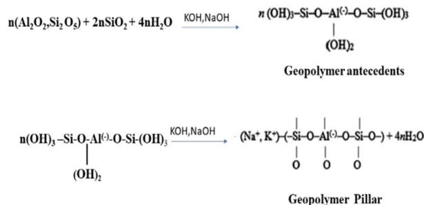
Fig. 13 Diagram showing polymerization process.<sup>1,87</sup>
