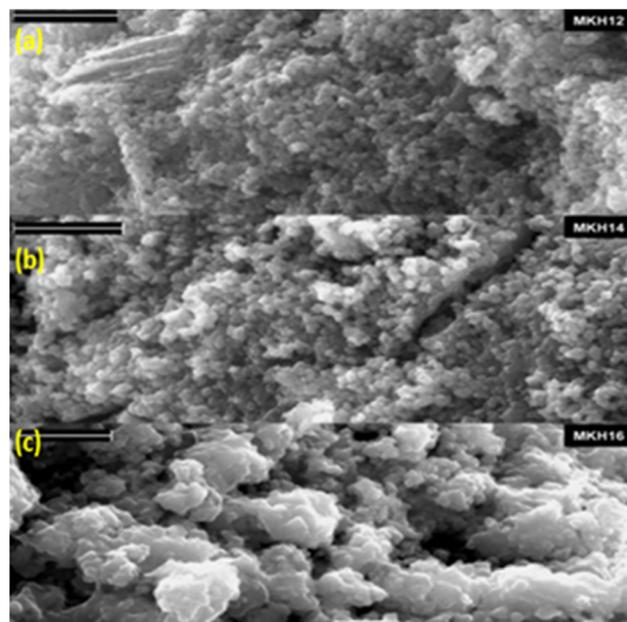
Fig. 34 (a)–(c) SEM images of metakaolin geopolymer at different H<sub>2</sub>O/Al<sub>2</sub>O<sub>3</sub> ratios; MKH represents H<sub>2</sub>O/Al<sub>2</sub>O<sub>3</sub> (a) 12, (b) 14 and (c) 16.<sup>71</sup>
