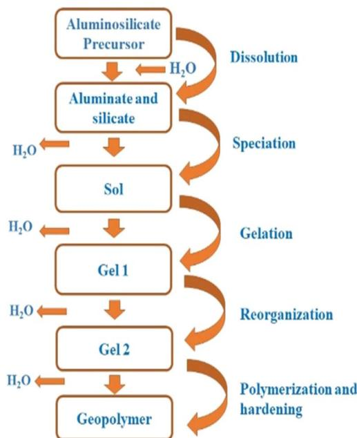
Fig. 14 Processes occurring during geopolymer formation.<sup>90,91</sup>
