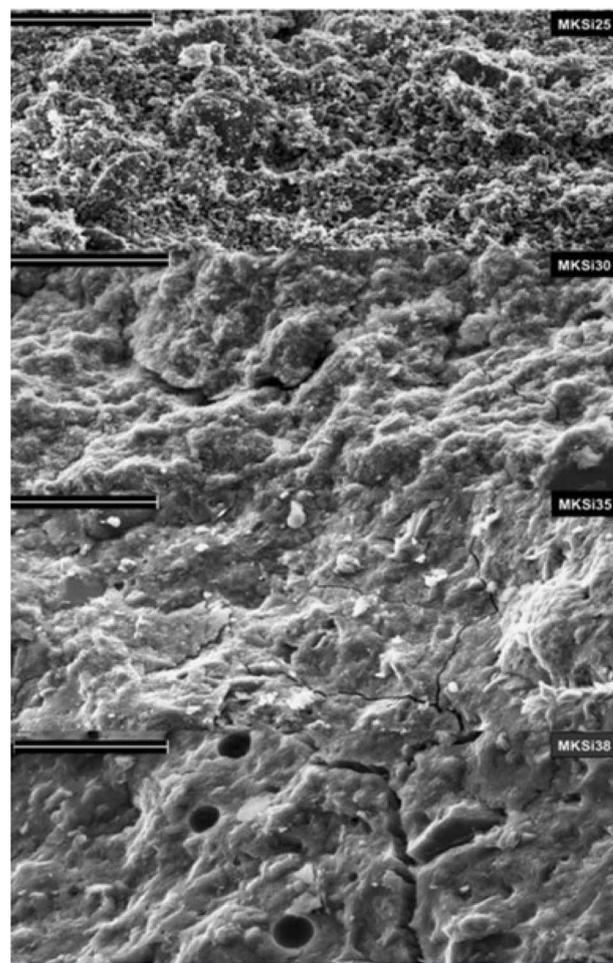
Fig. 16 SEM images show low porosity, high thickness, and fine-grained microstructures are factors that contribute to the formation of high-strength geopolymers.<sup>71</sup>
