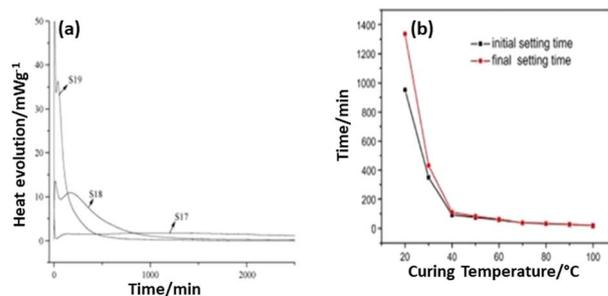
Fig. 38 (a) Effect of curing temperature on geopolymer reaction (S17 = 20 °C, S18 = 35 °C, S19 = 50 °C). (b) Effect of temperature on geopolymer reaction and setting time.<sup>38,163</sup>
