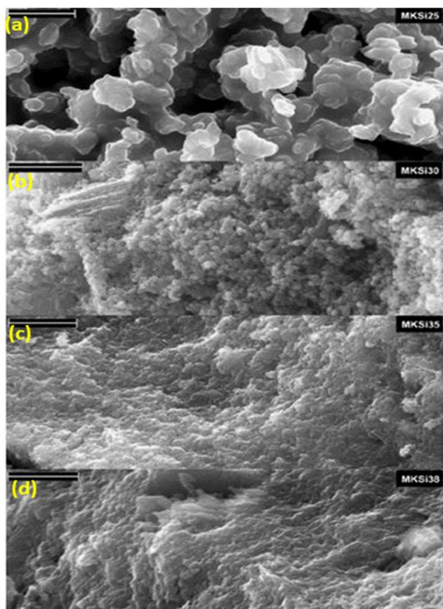
Fig. 31 (a)–(d) High-resolution SEM micrographs of metakaolin with different silica contents (MK = metakaolin, MKSi25– $\text{SiO}_2/\text{Al}_2\text{O}_3 = 2.5$ , MKSi30– $\text{SiO}_2/\text{Al}_2\text{O}_3 = 3.0$ , MKSi35– $\text{SiO}_2/\text{Al}_2\text{O}_3 = 3.5$ , and MKSi38– $\text{SiO}_2/\text{Al}_2\text{O}_3 = 3.8$ ).<sup>71</sup>
