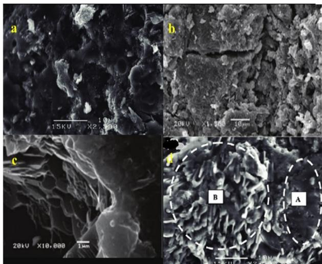
Fig. 5 SEM images of (a)–(c) pure metakaolin and (d) metakaolin geopolymer with slag where (“A” shows geopolymer matrix and “B” shows CSH gel).<sup>6</sup>
