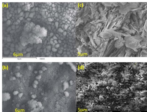
Fig. 8 SEM images of (a) and (b) kaolin made with NaOH solution and (c) and (d) kaolin made with alkaline sodium silicate solution.<sup>76,77</sup>
