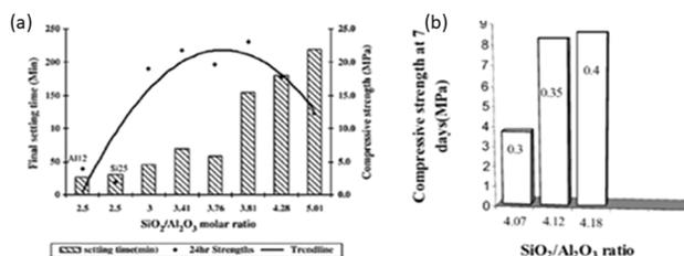
Fig. 23 (a) Compressive strength and final setting time of metakaolin geopolymer with constant H<sub>2</sub>O/Na<sub>2</sub>O molar ratio of 13.6 and varying SiO<sub>2</sub>/Al<sub>2</sub>O<sub>3</sub> ratios. (b) Compressive strength of geopolymer with varying SiO<sub>2</sub>/Al<sub>2</sub>O<sub>3</sub> ratios.<sup>37,120</sup>
