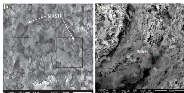
Fig. 25 (a) SEM image of fly ash-based geopolymer exposed to acid attack for 365 days. (b) SEM image of kaolinite geopolymer exposed to acid attack for 90 days.<sup>126,127</sup>
