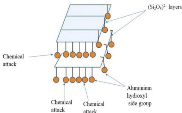
Fig. 11 Chemical attack on kaolinite layers (orange circles represent aluminium hydroxyl side group).<sup>6</sup>
