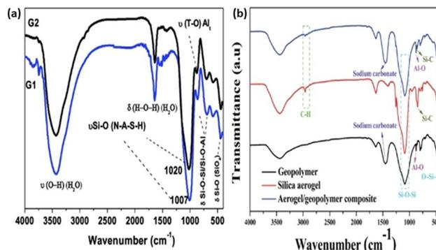
Fig. 22 (a) FTIR spectra of (G1 = Gel 1) and (G2 = Gel 2). (b) FTIR spectra of geopolymer, aerogel/geopolymer composite and aerogel.<sup>115,116</sup>
