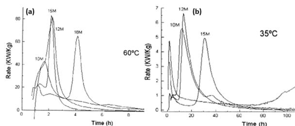
Fig. 27 (a) Calorimetric curves of calcium hydroxide used with metakaolin geopolymer. (b) Curves showing heat evolution of geopolymer activated with NaOH solution.<sup>61</sup>
