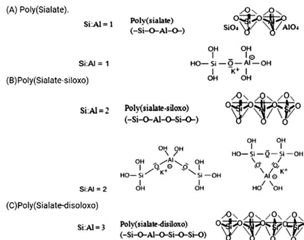
Fig. 2 (A)–(C) Various geopolymer systems based on the Si : Al ratio.<sup>8–10</sup>
