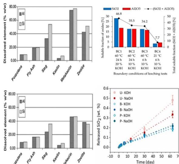
Fig. 6 Aluminium (Al) and silicon (Si) were dissolved in 10% 10 M NaOH and KOH solutions, respectively. The soluble fraction of oxides and the total soluble fraction of oxides of metakaolin were analyzed. Additionally, the release of  $\text{SiO}_2$  from different aggregates in 0.4 M NaOH and KOH solutions was measured as a function of time at 38 °C.<sup>68–70</sup>
