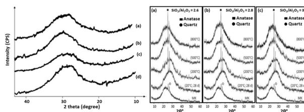
Fig. 20 (Left side panel) XRD diffractograms for poly(sialate-siloxo) geopolymers with molar ratios of  $\text{SiO}_2/\text{Al}_2\text{O}_3$  of (a) 4.02; (b) 3.98; (c) 3.39; and (d) 4.11. (Right) (a)–(c) XRD diffractograms of geopolymers with different  $\text{SiO}_2/\text{Al}_2\text{O}_3$  ratios and cured at different temperatures.<sup>104,105</sup>
