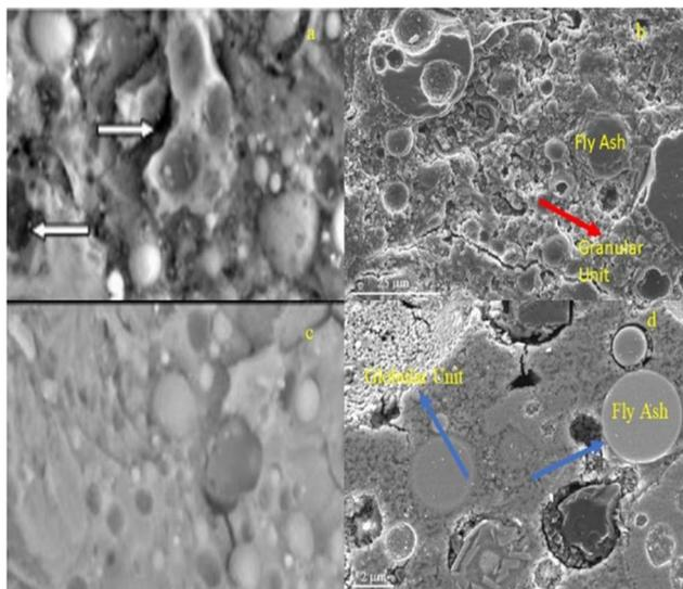
Fig. 10 SEM images of fly-ash-based geopolymers made with (a)–(c) NaOH solution and (d) alkaline silicate solution.<sup>78–80</sup>
