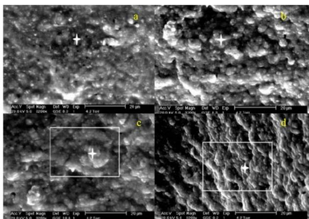
Fig. 18 ESEM micrographs obtained for the same area at different mixing times of (a) 10 min, (b) 3 h, (c) 6 h and (d) 9 h.<sup>86,100,103</sup>
