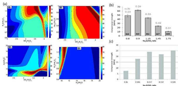
Fig. 35 (a) Effect of various molar ratios ( $R_2O/Al_2O_3$ ,  $SiO_2/Al_2O_3$ ,  $Na_2O/K_2O$  and  $H_2O/R_2O$ ), where ( $R = Na$  or  $K$ ) on the compressive strength of metakaolin geopolymers shown in a contour plot. The units of contour are in MPa. (b) Graph showing the effect of  $Na_2O/Al_2O_3$  molar ratio on the compressive strength of a geopolymer. (c) Graph showing the effect of  $Na_2O/SiO_2$  molar ratio on the compressive strength of a geopolymer.<sup>157–159</sup>
