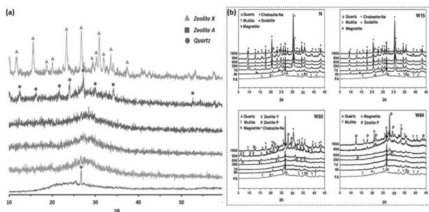
Fig. 33 (a) XRD patterns of metakaolin geopolymer made with different SiO<sub>2</sub>/Na<sub>2</sub>O ratios of 2.25, 2.50, 3.00, 3.50, 4.00, and XRD pattern of metakaolin. (b) XRD patterns of fly ash geopolymer with different SiO<sub>2</sub>/Na<sub>2</sub>O ratios, for N, W15, W50 and W84 the SiO<sub>2</sub>/Na<sub>2</sub>O values are 0, 0.19, 0.69, and 1.17, respectively.<sup>112,153</sup>
