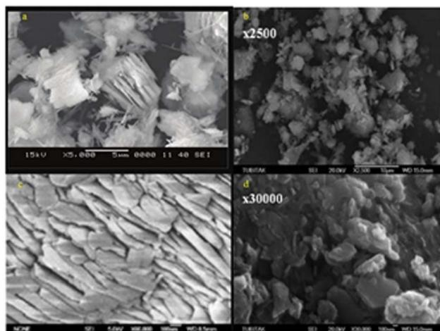
Fig. 4 (a)–(d) SEM micrographs of metakaolin calcined at different temperatures.<sup>6,43,44</sup>
