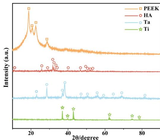
Fig. 12 XRD patterns of plasma sprayed Ta, HA, Ti coatings and PEEK plate scaffold.
