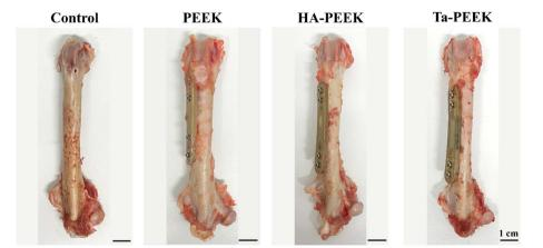
Fig. 15 Appearance of rabbit femur after 12 weeks of implantation of different bioactive bone plate scaffolds.
