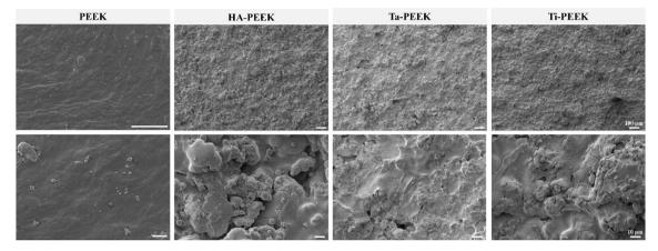
Fig. 10 The SEM images of PEEK, HA-PEEK, Ta-PEEK and Ti-PEEK bone plate scaffold
