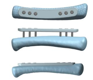
Assembly of plate scaffold model and screw model.
