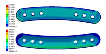
Fig. 8 Stress distribution of bone plate scaffold in finite element
