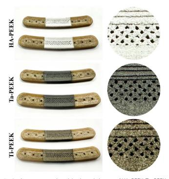
Fig. 9 Appearance and partial enlarged pictures of HA-PEEK, Ta-PEEK and Ti-PEEK plate scaffolds.
