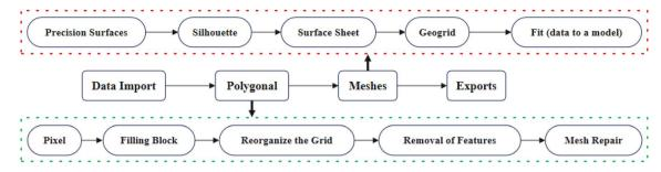
Fig. 1 Surface treatment process of rabbit femur model.
