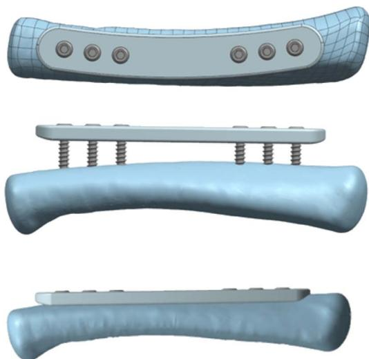
Fig. 7 Assembly of plate scaffold model and screw model.
