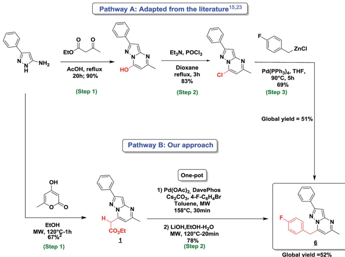
Scheme 17 Comparison between the literature method and this study's synthesis.<sup>84</sup>
