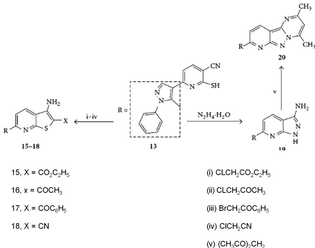
Scheme 10 Synthesis of thieno[2,3-*b*]pyridines (15–18) and pyrido[2',3':3,4]pyrazolo[1,5-*a*]pyrimidine (20).<sup>65</sup>
