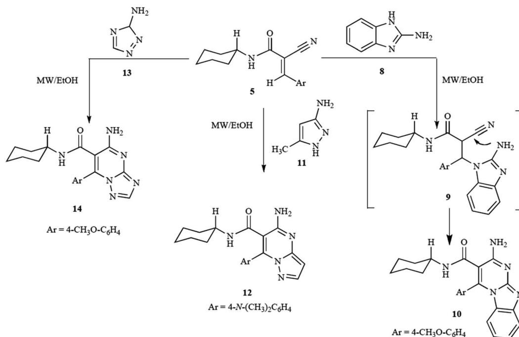
Scheme 16 Synthesis of pyrazolo[1,5-*a*]pyrimidines and pyrazolo[1,5-*a*]quinazolines.<sup>82</sup>
