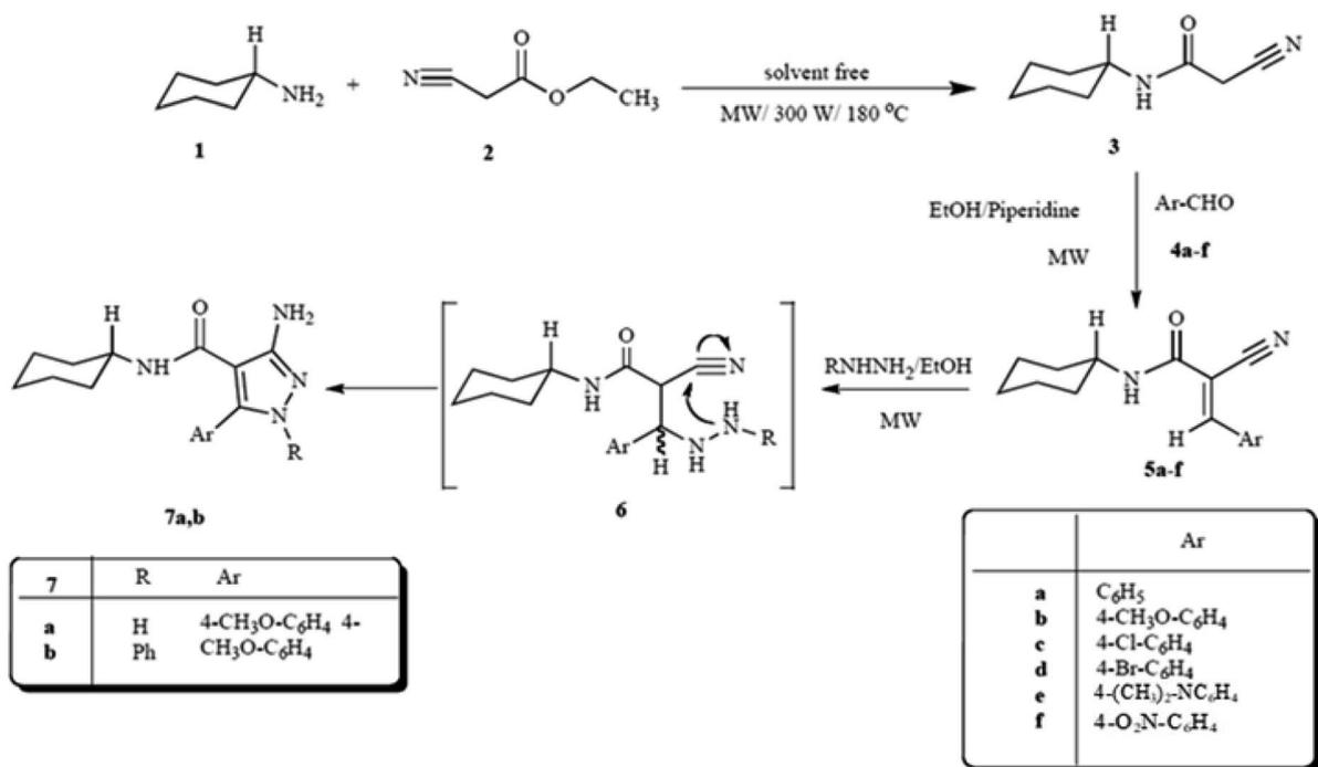
Scheme 14 Synthesis of 2-cyano-*N*-cyclohexylacetamide (**3**), followed by its reaction with aromatic aldehyde derivatives and the subsequent reaction of acrylamide derivatives with hydrazine derivatives.<sup>81</sup>
