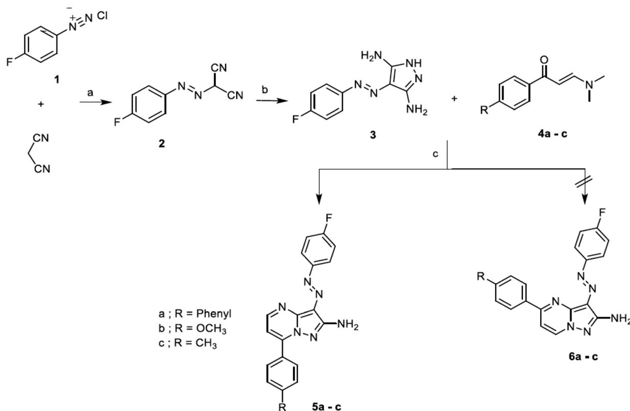
**Scheme 28** The preparation of 3-((4-fluorophenyl)diazonyl)-7-(4-substituted phenyl)pyrazolo[1,5-*a*]pyrimidin-2-amine **5a–c**. Reagents and condition: (a) sodium acetate/EtOH, stirring for 30 min/cooling. (b) NH<sub>2</sub>NH<sub>2</sub>·H<sub>2</sub>O/EtOH, reflux 6 h. (c) GL acetic acid, reflux 7 h.
