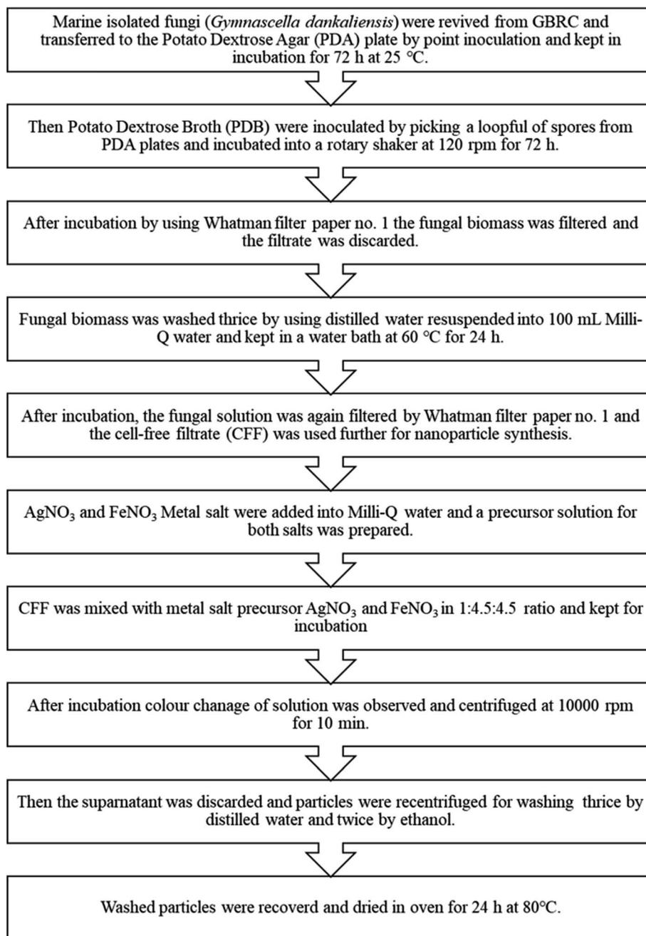
Fig. 1 Flow chart of the methodology for AgFe-BMNPs synthesis.
