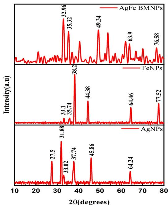
Fig. 3 Diffractogram of AgFe-BMNPs, Ag, and FeNPs.
