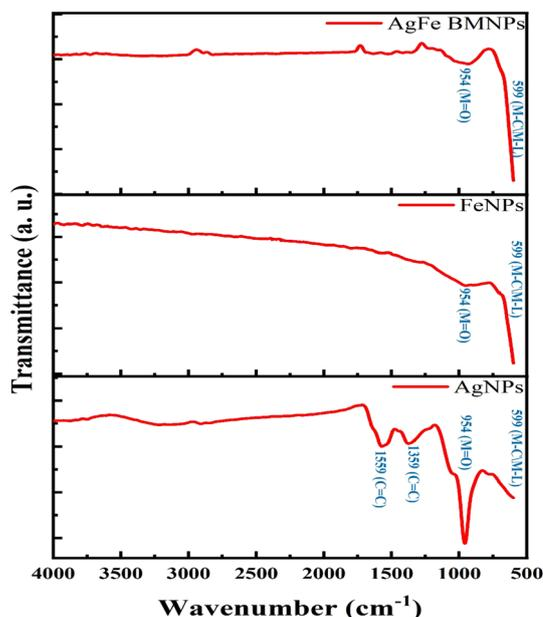
Fig. 4 FTIR spectrum for AgFe-BMNPs, Ag, and FeNPs.
