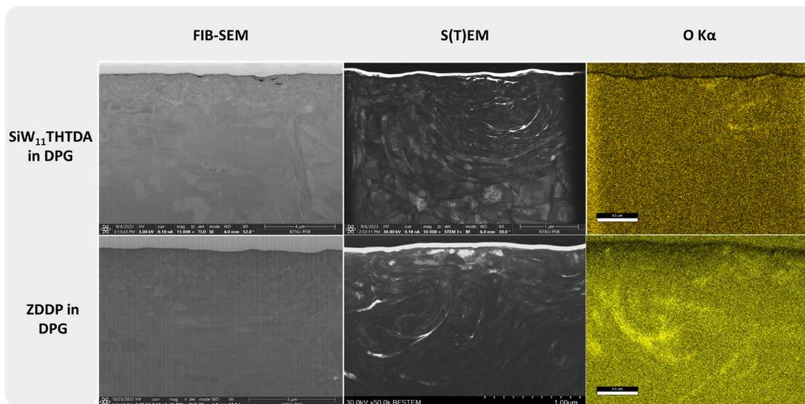
Fig. 4 Cross section images and elemental mapping of the wear tracks of SiW<sub>11</sub>THTDA and ZDDP in DPG.
