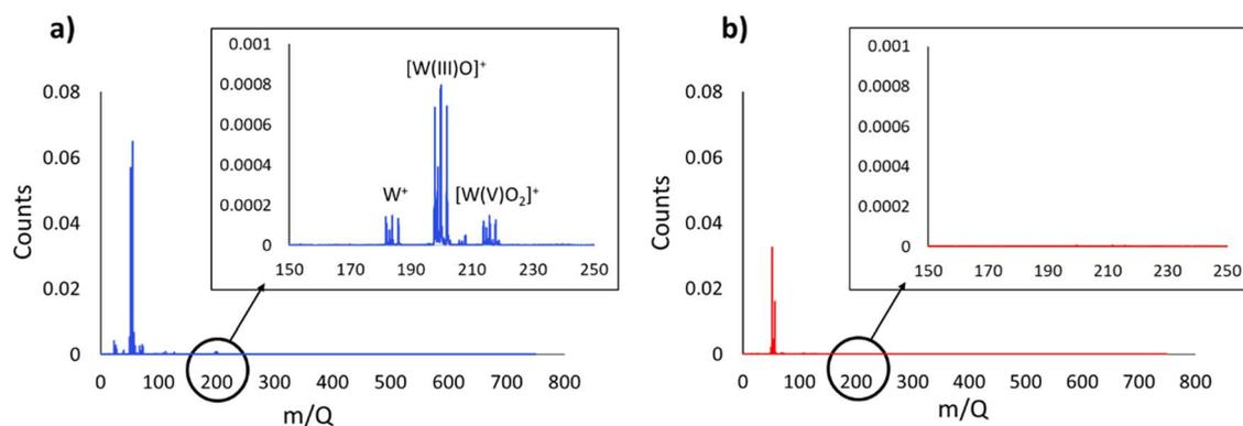
Fig. 7 ToF-SIMS analysis of (a) inside and (b) outside the wear track of SiW<sub>11</sub>THTDA in PAO8.
