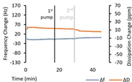
Fig. 6 QCM-D plots versus time, showing frequency change and dissipation for ZDDP at 0.01 wt% in PAO8.
