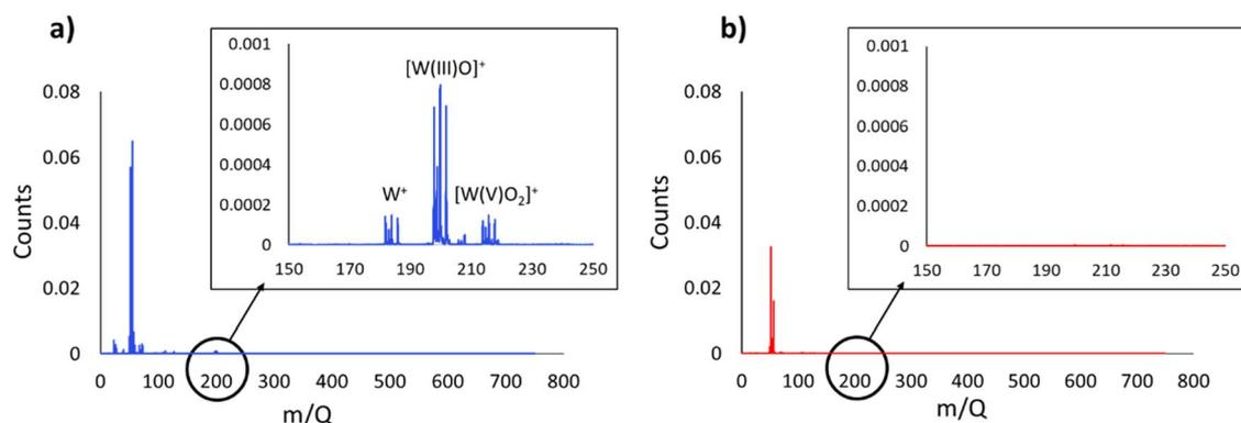
Fig. 7 ToF-SIMS analysis of (a) inside and (b) outside the wear track of SiW<sub>11</sub>THTDA in PAO8.
