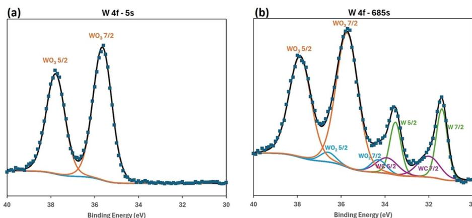
Fig. 8 XPS analysis inside the wear track of SiW<sub>11</sub>THTDA in PAO8 showing the presence of tungsten at (a) 5 seconds and (b) 685 seconds etch time.
