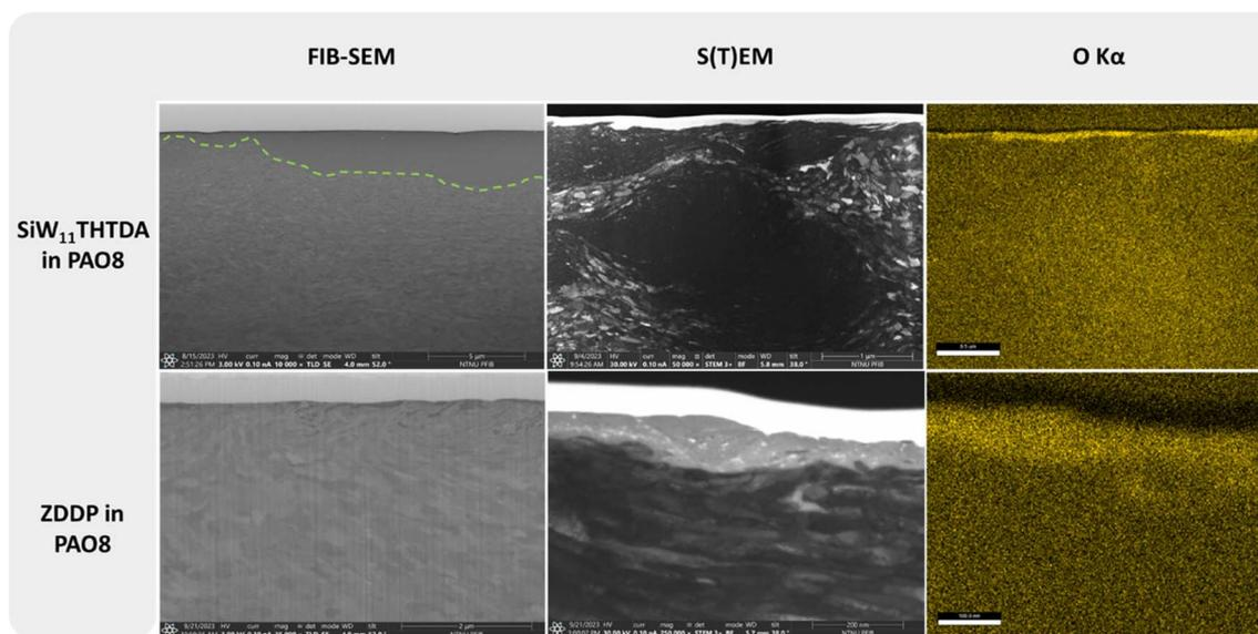
Fig. 3 Cross section images and elemental mapping of the wear tracks of SiW<sub>11</sub>THTDA and ZDDP in PAO8.
