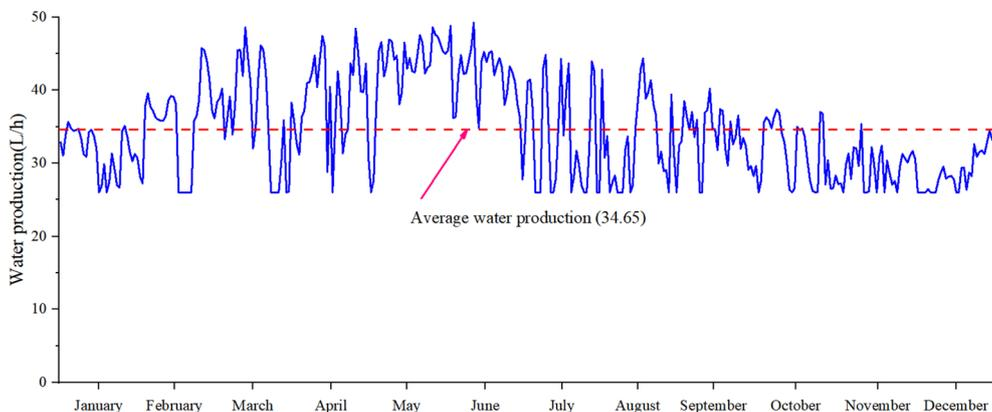
Fig. 8 Average water production based on increased membrane area.
