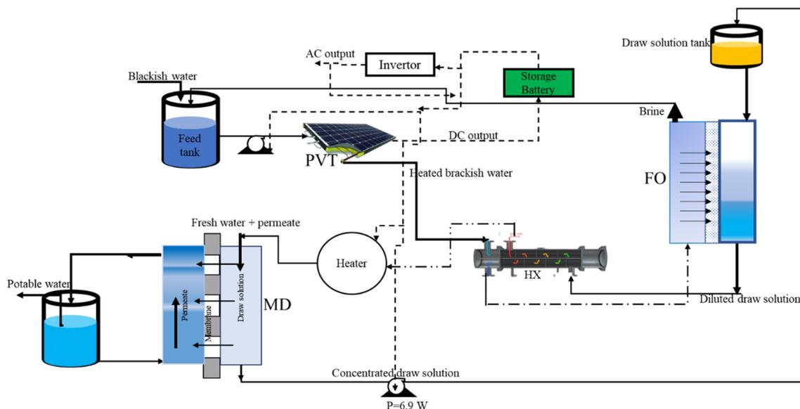
Fig. 1 PVT driven FO–MD desalination pilot unit.
