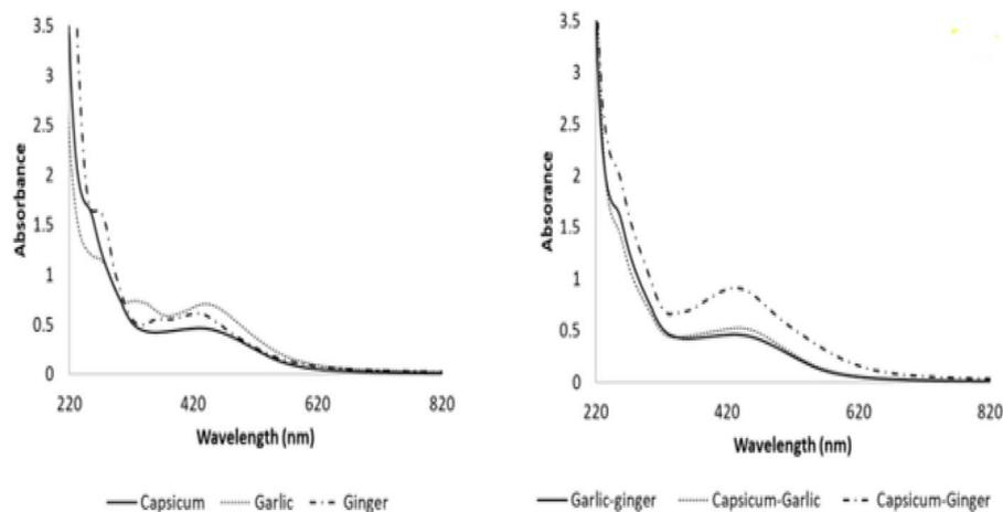
Fig. 6 UV-vis spectra of SNPs (left) extracts of pure plants, (right) extracts obtained from mixtures of plant extracts<sup>236</sup>
