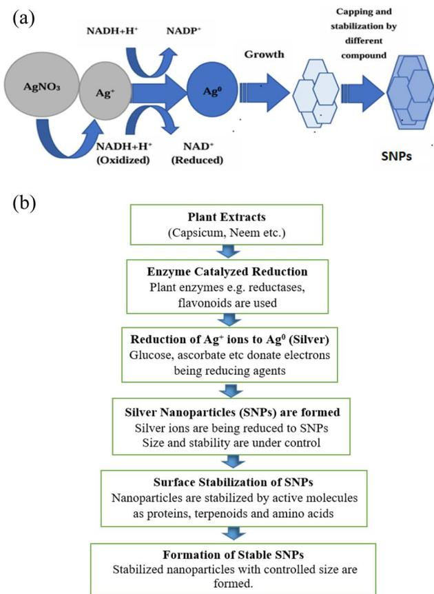
Fig. 5 (a) The supposed biosynthesis mechanism of SNPs.<sup>177</sup> (b) Flowsheet diagram showing mechanistic pathway of SNPs.
