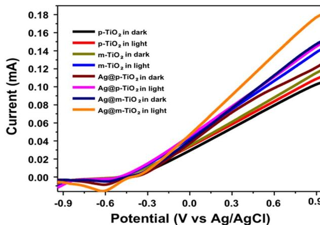
Fig. 11 Linear scan voltammograms of the *p*-TiO<sub>2</sub> and *m*-TiO<sub>2</sub> NPs as well as Ag@*p*-TiO<sub>2</sub> and Ag@*m*-TiO<sub>2</sub> nanocomposites photoelectrodes in the dark and under visible light irradiation.<sup>253</sup>
