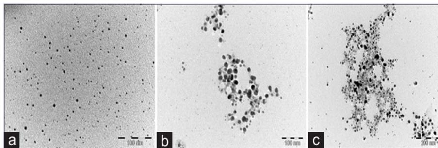
Fig. 8 Micrographs of SNPs taken through TEM (a) garlic, (b) ginger, and (c) cayenne pepper.<sup>244</sup>
