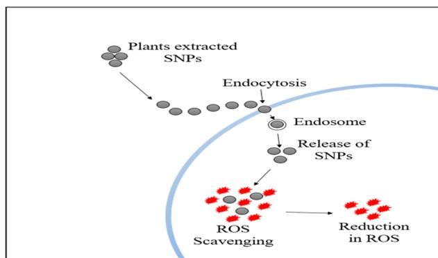
Fig. 17 Radical oxygen scavenging mechanism.<sup>266</sup>
