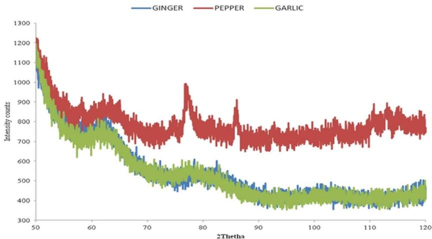
Fig. 10 XRD of SNPs obtained by using garlic, ginger, and cayenne pepper<sup>244</sup>
