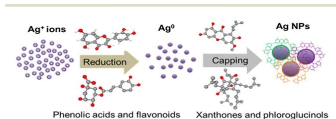
Fig. 4 Reduction and capping of SNPs<sup>167</sup>
