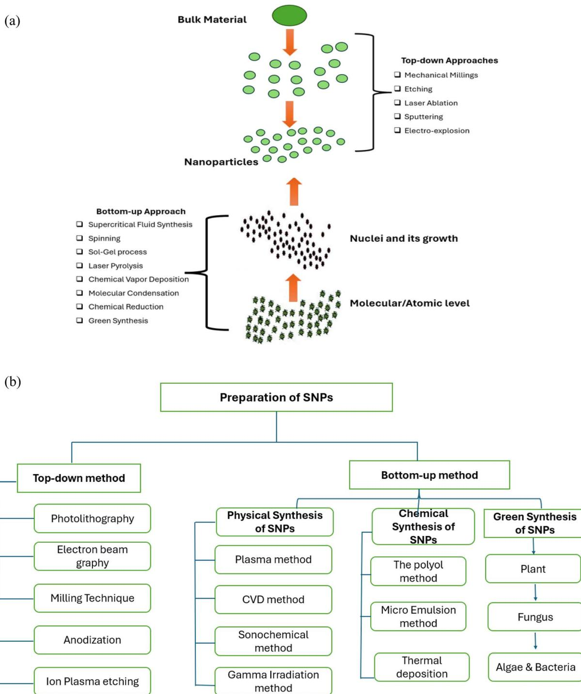
Fig. 1 (a) Methods for producing NPs.<sup>29</sup> (b) Enlisting the conventional and green synthesis methods of SNPs (reconstructed and modified from ref. 30).
