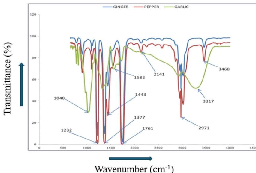
Fig. 9 FTIR spectra of SNPs from garlic, ginger, and cayenne pepper<sup>244</sup>
