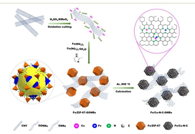
Scheme 1 Schematic for the synthesis of Fe/Co-N-C-GNRs hybrids.
