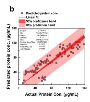
Fig. 6 A scatterplot showing the difference between BCA assay (a), Bradford assay (b), the predicted protein concentration for the test (Y-axis) and observed protein concentration (X-axis) set based on the linear model. Linear regression plot with 95% confidence intervals (shaded areas) showing the predicted relationship between predicted and observed protein concentration.
