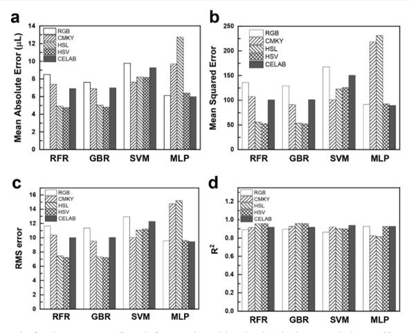
Fig. 5 Bar graphs of metric scores corresponding to the four regression models, each evaluated against a mean absolute error (a), mean squared error (b), root mean squared error (c), and  $R^2$  (d) dataset represented in five distinct color systems.
