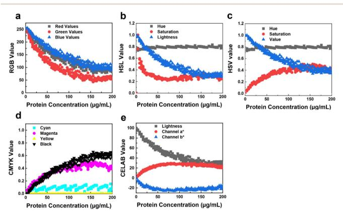
Fig. 2 Scatter color data plots illustrating the distribution of values for each color channel across five distinct colorimetry models, applied to a dataset of protein extracted from 96 well plates where the BCA protein assay was conducted. RGB (a), HSL (b), HSV (c), CMYK (d), and CIELAB (e) values from five assays.
