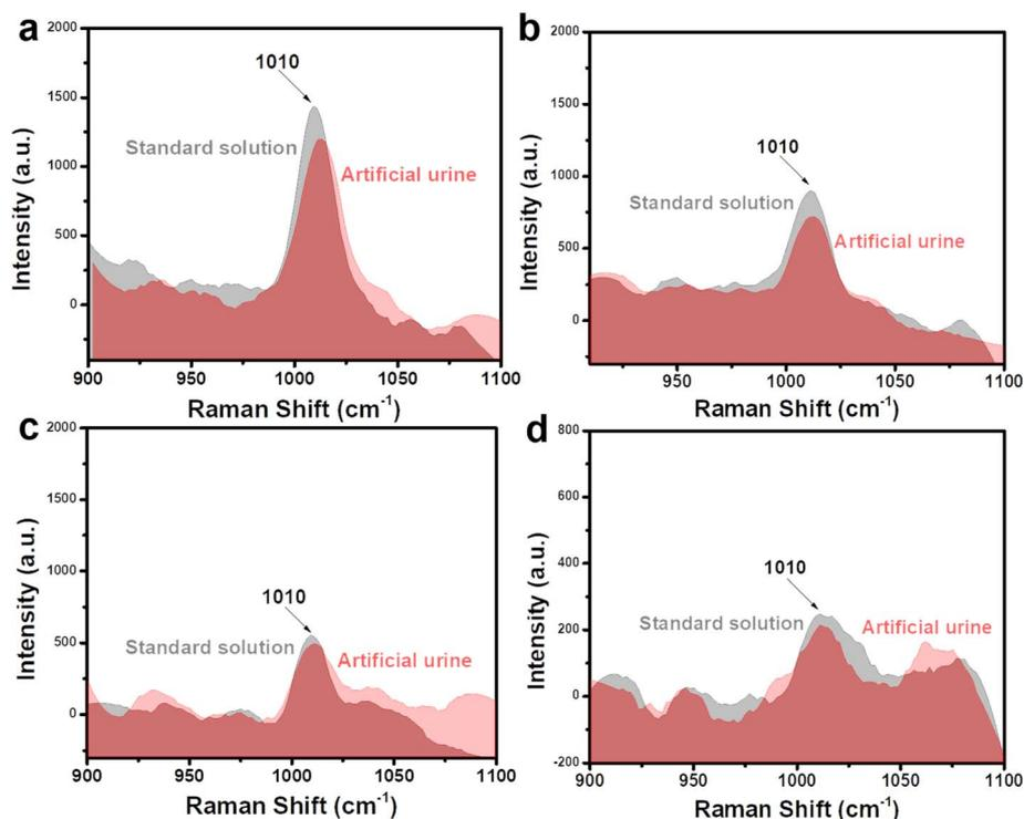
Fig. 7 Comparison of SERS signals of urea obtained from artificial urine sample with the standard solution at concentrations of  $10^{-5}$  M (a),  $10^{-6}$  M (b),  $10^{-7}$  M (c), and  $10^{-8}$  M (d).
