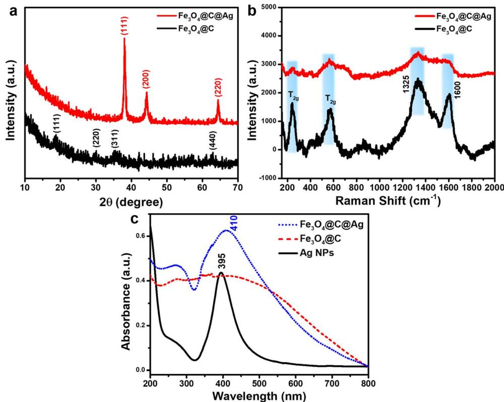
Fig. 3 XRD patterns (a), Raman spectra (b) and UV-Vis spectra (c) of  $\text{Fe}_3\text{O}_4@\text{C}$  and  $\text{Fe}_3\text{O}_4@\text{C}@\text{Ag}$ .
