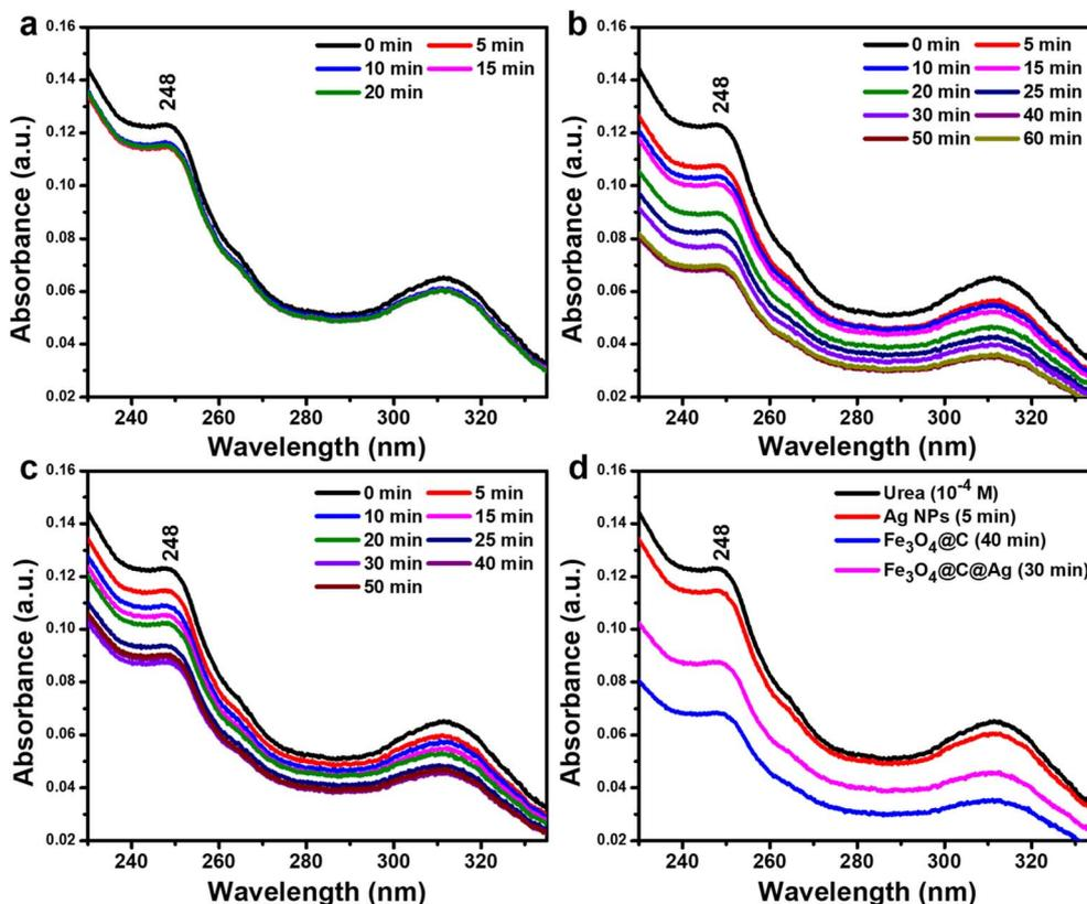
Fig. 4 Evaluation of urea adsorption over time by monitoring the decrease in the intensity of the characteristic absorption peak at 248 nm for Ag NPs (a), Fe<sub>3</sub>O<sub>4</sub>@C (b), and Fe<sub>3</sub>O<sub>4</sub>@C@Ag (c). The comparison highlights the adsorption efficiency of urea across these materials at their respective equilibrium adsorption points (d).
