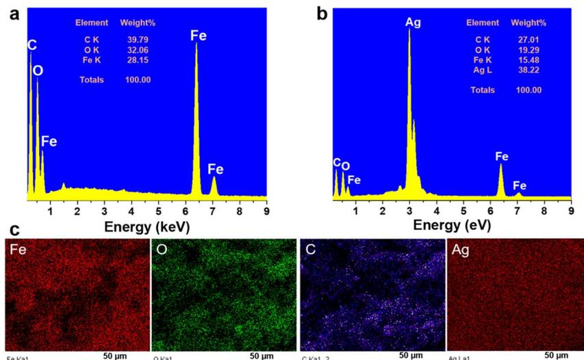
Fig. 2 EDX spectra of Fe<sub>3</sub>O<sub>4</sub>@C (a) and Fe<sub>3</sub>O<sub>4</sub>@C@Ag (b); and EDX mapping analysis of Fe<sub>3</sub>O<sub>4</sub>@C@Ag (c).
