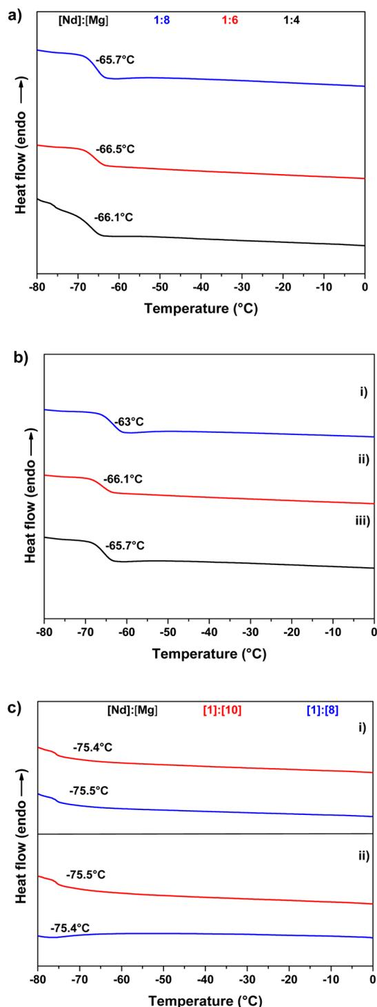
Fig. 5 Thermograms of polymerized terpenes: (a)  $\beta$ -myrcene polymerized at 50 °C with varying  $[\text{Nd}] : [\text{Mg}]$  ratios. (b)  $\beta$ -Myrcene polymerized at varying temperatures: (i) 70 °C, (ii) 60 °C and (iii) 50 °C. (c)  $\beta$ -Farnesene polymerized at (i) 60 °C and (ii) 70 °C with varying  $[\text{Nd}] : [\text{Mg}]$  ratios.
