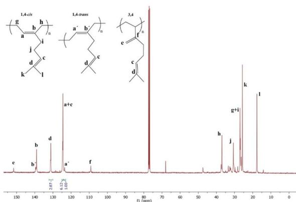
Fig. 4  $^{13}\text{C}$  NMR spectra, corresponding to Run My2, in order to illustrate the signal assignment in a polymyrcene sample.
