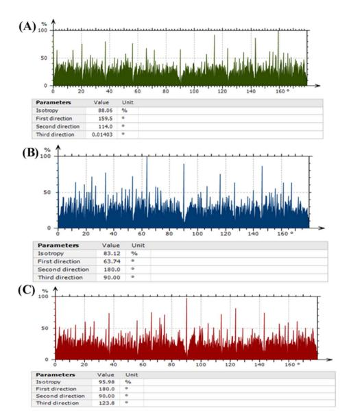
Fig. 7 Cartesian graphs of the surface texture directions for (A) PANI, (B) CB, and (C) PANI/CB.
