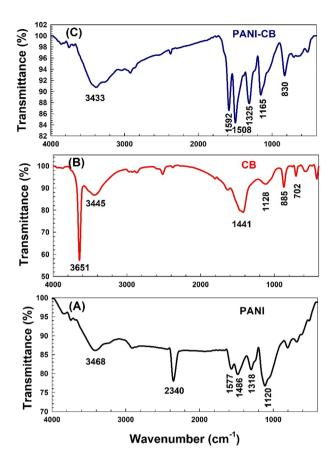
Fig. 4 FTIR spectrum of (A) PANI (B) CB (C) PANI/CB.
