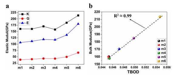
Fig. 9 (a) The distribution of Young's modulus (E), bulk modulus (E), and shear modulus (E) for the 6 BCC RHEAs. (b) Illustrates the relationship between total bond order density (TBOD) and the bulk modulus (E) for the same set of 6 BCC RHEAs.
