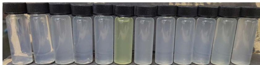
Fig. 13 Solution of AE-3 (10  $\mu\text{M}$ ) with different metal ions (10  $\mu\text{M}$ ) in THF/phosphate buffer (1/9, v/v, 50 mM, pH = 7.4) incubated for 10 min and observed in daylight. From left to right, the sequence is:  $\text{Fe}^{3+}$ ,  $\text{Al}^{3+}$ ,  $\text{Cd}^{2+}$ ,  $\text{Mg}^{2+}$ ,  $\text{Cu}^{2+}$ ,  $\text{Co}^{2+}$ ,  $\text{Ba}^{2+}$ ,  $\text{Ca}^{2+}$ ,  $\text{Cr}^{3+}$ ,  $\text{Mn}^{2+}$ ,  $\text{Ni}^{2+}$ , and  $\text{Zn}^{2+}$ .
