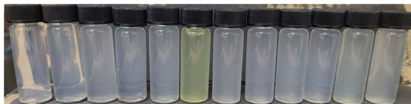
Fig. 13 Solution of AE-3 (10 \mu\text{M} ) with different metal ions (10 \mu\text{M} ) in THF/phosphate buffer (1/9, v/v, 50 mM, pH = 7.4) incubated for 10 min and observed in daylight. From left to right, the sequence is: \text{Fe}^{3+} , \text{Al}^{3+} , \text{Cd}^{2+} , \text{Mg}^{2+} , \text{Cu}^{2+} , \text{Co}^{2+} , \text{Ba}^{2+} , \text{Ca}^{2+} , \text{Cr}^{3+} , \text{Mn}^{2+} , \text{Ni}^{2+} , and \text{Zn}^{2+} .
