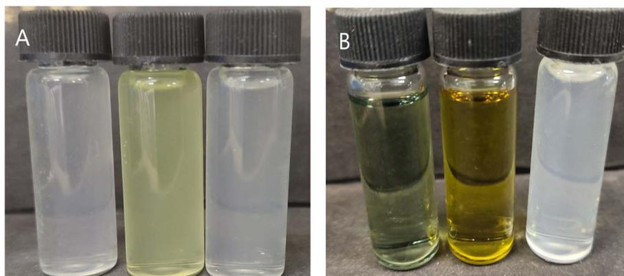
Fig. 14 (A) Solution of AE-3 (10  $\mu\text{M}$ ) with HClO and  $\text{Co}^{2+}$  (10  $\mu\text{M}$ ) in THF/phosphate buffer (1/9, v/v, 50 mM, pH = 7.4) incubated for 10 min and observed in daylight. (B) Solution of AE-3 (500  $\mu\text{M}$ ) with HClO and  $\text{Co}^{2+}$  (100  $\mu\text{M}$ ) in THF/phosphate buffer (1/4, v/v, 50 mM, pH = 7.4) incubated for 10 min and observed in daylight. From left to right, they are HClO,  $\text{Co}^{2+}$  and blank samples.
