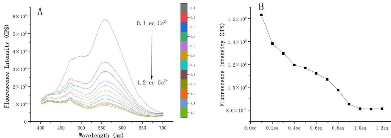
Fig. 17 (A) Fluorescence spectra of AE-3 (10  $\mu\text{M}$ ) with the addition of 0.1–1.2 eq.  $\text{Co}^{2+}$  in THF/phosphate buffer (1/9, v/v, 50 mM, pH = 7.4). (B) Relationship of AE-3 (10  $\mu\text{M}$ ) fluorescence intensity at 556 nm and  $\text{Co}^{2+}$  equivalents in the THF/phosphate buffer (1/9, v/v, 50 mM, pH = 7.4).
