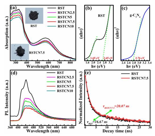
Fig. 4 Optical properties and carrier kinetics of different samples. (a) Absorption spectra of different samples.  $E_g$  values for (b) pure RST, (c) g- $C_3N_4$  (d) PL spectra of different samples, (e) PL-decay of RST and RSTCN7.5.
