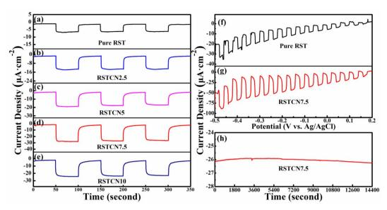
Fig. 3 PEC properties of different samples. Photocurrent versus time under chopped light (a) pure RST, (b) RSTCN2.5, (c) RSTCN5, (d) RSTCN7.5 and (e) RSTCN10. LSV curves under chopped light (f) pure RST and (g) RSTCN7.5 sample. (h) Longtime photocurrent versus time under light for 4 hours of RSTCN7.5 sample.
