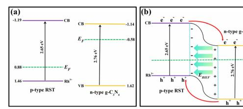
Fig. 7 Energy diagram for enhanced PEC performance. (a) Band edges position between RST and  $g-C_3N_4$  before contact, (b) band alignment between RST and  $g-C_3N_4$  after contact ( $E_{BIEF}$ : built-in electric field).
