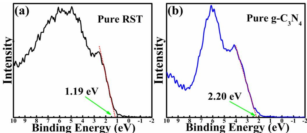
Fig. 6 XPS valence band spectra of different samples. (a) RST and (b)  $g\text{-C}_3\text{N}_4$ .
