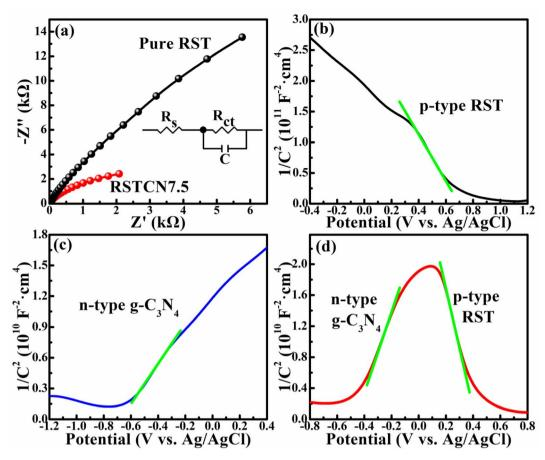
Fig. 5 (a) EIS of RST and RSTCN7.5 samples. Mott–Schottky curves of different samples. (b) RST, (c) g-C<sub>3</sub>N<sub>4</sub>, and (d) RSTCN7.5 heterojunction.
