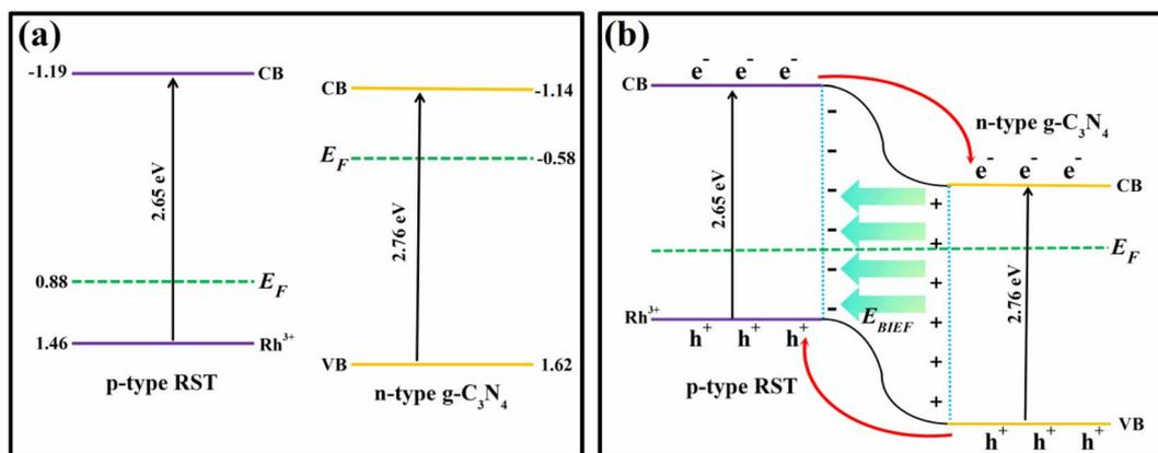
Fig. 7 Energy diagram for enhanced PEC performance. (a) Band edges position between RST and  $g\text{-C}_3\text{N}_4$  before contact, (b) band alignment between RST and  $g\text{-C}_3\text{N}_4$  after contact ( $E_{BIEF}$ : built-in electric field).
