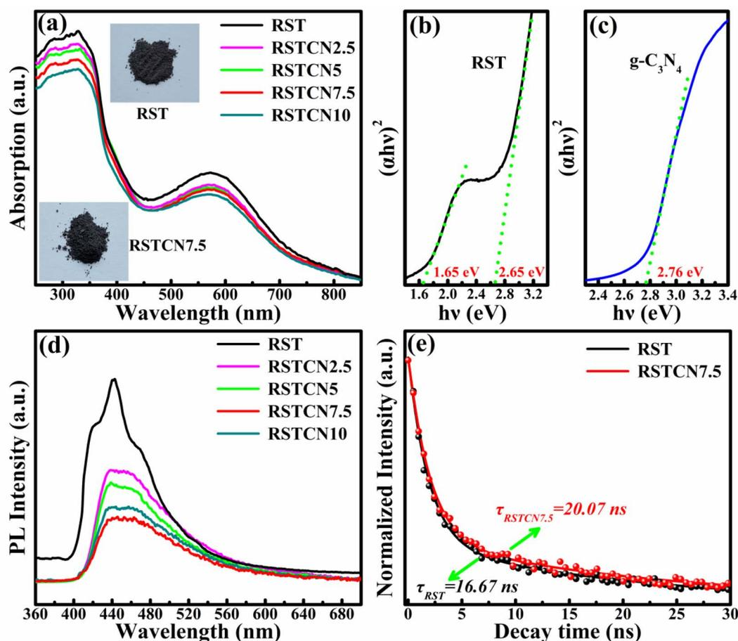
Fig. 4 Optical properties and carrier kinetics of different samples. (a) Absorption spectra of different samples.  $E_g$  values for (b) pure RST, (c)  $g\text{-C}_3\text{N}_4$ . (d) PL spectra of different samples, (e) PL-decay of RST and RSTCN7.5.
