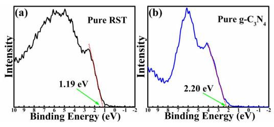
Fig. 6 XPS valence band spectra of different samples. (a) RST and (b) g-C<sub>3</sub>N<sub>4</sub>.
