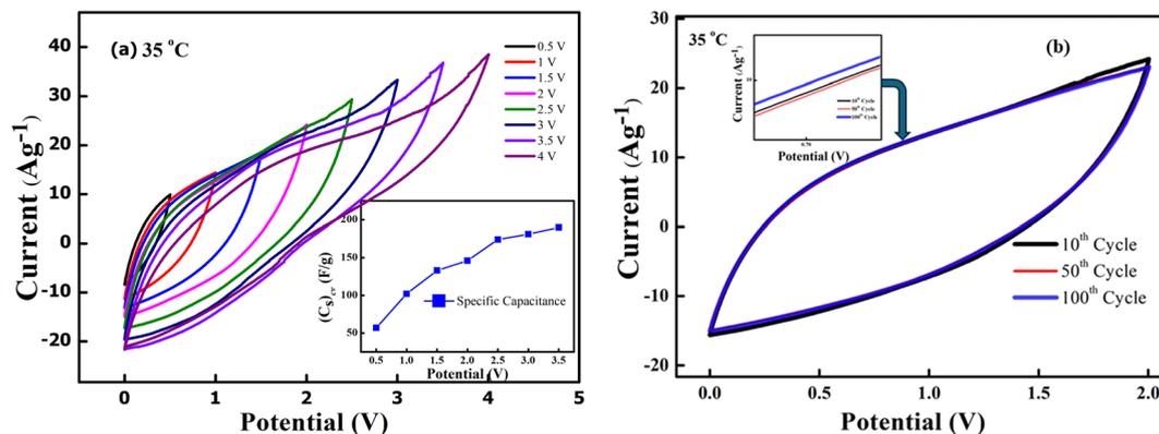
Fig. 10 (a) CV scans ( $100 \text{ mV s}^{-1}$ ) of SSC for different voltage range at  $35 \text{ }^\circ\text{C}$ . (Inset) Variation of specific capacitance ( $C_{s,CV}$ ) with operating potential. (b) 100 cycles of CV scan ( $100 \text{ mV s}^{-1}$ ) at  $2 \text{ V}$  and  $35 \text{ }^\circ\text{C}$ .
