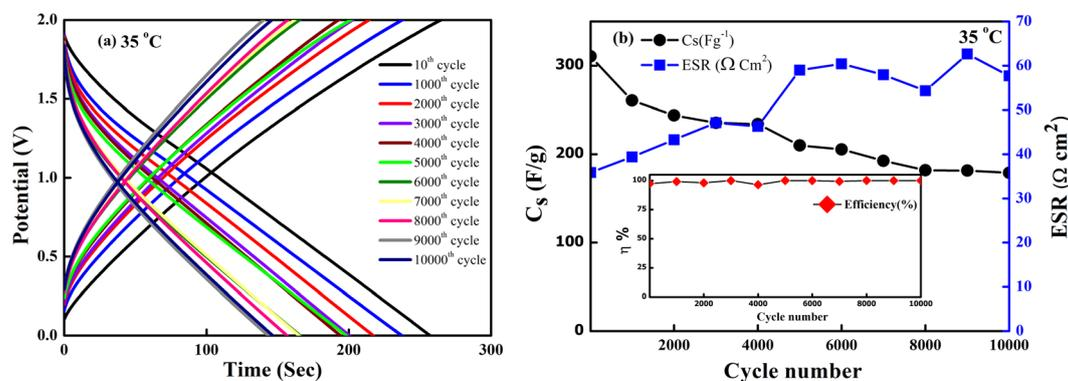
**Fig. 13** (a) Charge-discharge curves obtained at different cycles for SSC with LLTO-6% EMIM BF<sub>4</sub> composite as electrolyte at room temperature. (b) Specific capacitance and ESR vs. cycle number at room temperature for SSC having electrolyte LLTO-6% EMIM BF<sub>4</sub>. Inset shows coulombic efficiency vs. cycle number up to  $10\,000$  cycles.
