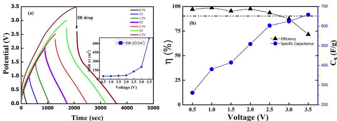
Fig. 11 (a) GCD curves to obtain the cutoff voltage at  $1 \text{ mA}$  discharge current for different potential. (Inset) Nature of ESR with potential (b) coulombic efficiency of the SSC with its specific capacity.
