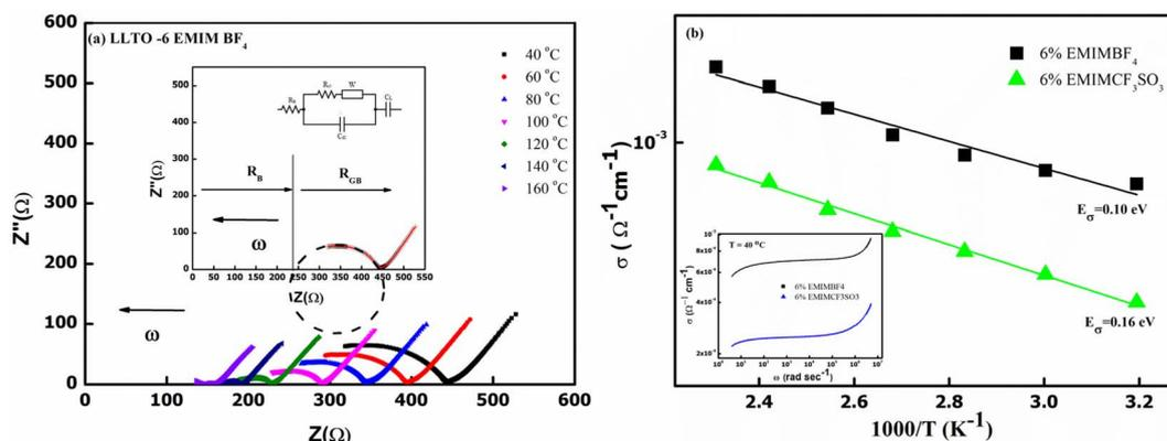
Fig. 8 (a) Nyquist plot of the LLTO–6 EMIM BF<sub>4</sub> with the equivalent circuit in the inset. (b) Total conductivity of LLTO with different IL. (Inset) Frequency dependence of the electrical conductivity of both LLTO–IL composite at 40 °C.
