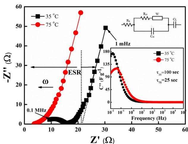
Fig. 9 The Nyquist plot and corresponding equivalent circuit for the laminated geometry at two different temperatures having LLTO–6 EMIM BF<sub>4</sub> composite as an electrolyte. (Inset) Imaginary capacitance ( $C''$ ) vs. frequency (Hz).
