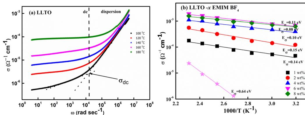
Fig. 7 (a) Frequency dependence of electrical conductivity for pristine LLTO (b) temperature dependence of total conductivity for all the composites having LLTO and varied amount of EMIM BF<sub>4</sub>.
