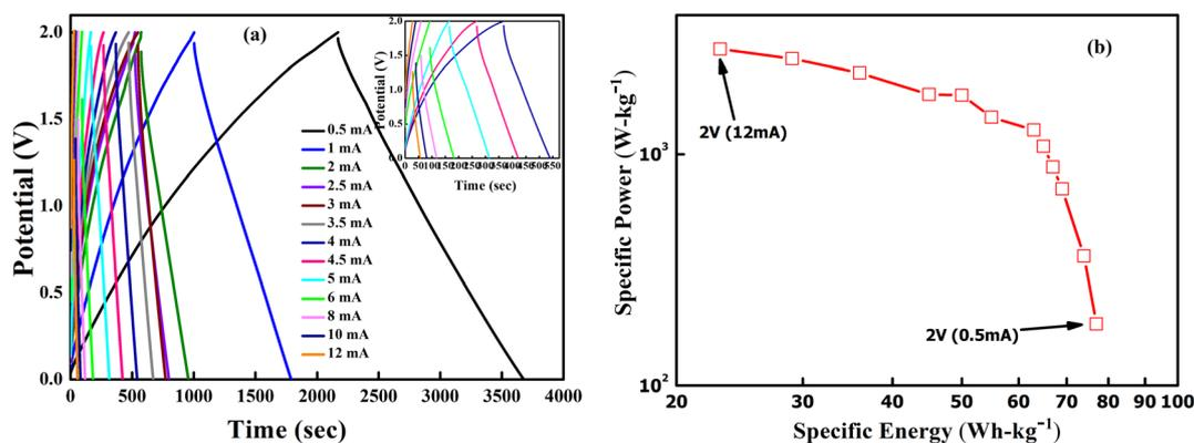
**Fig. 12** (a) GCD curves of LLTO-6% EMIM BF<sub>4</sub> for the 10th cycle at different discharge currents ranging from  $0.5\text{ mA}$  to  $12\text{ mA}$ . (b) Ragone plot for SSC at  $0\text{--}2\text{ V}$  range.
