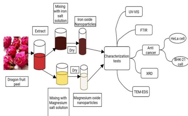
Fig. 1 Schematic of the biosynthesis of the nanoparticles and their characterization tests.
