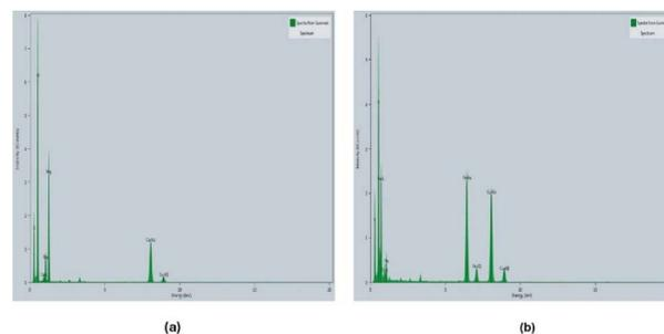
Fig. 10 EDX spectrum of (a) Fe<sub>2</sub>O<sub>3</sub> NPs and (b) MgONPs.
