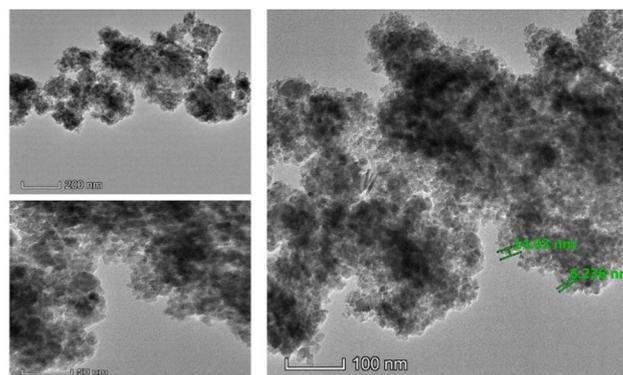
Fig. 8 TEM images of Fe<sub>2</sub>O<sub>3</sub> NPs.
