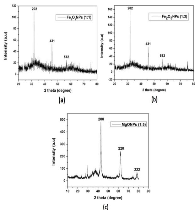
Fig. 7 XRD spectra of nanoparticles: (a) Fe<sub>2</sub>O<sub>3</sub>NPs (1 : 1), (b) Fe<sub>2</sub>O<sub>3</sub>NPs (1 : 3) and (c) MgONPs (1 : 5).
