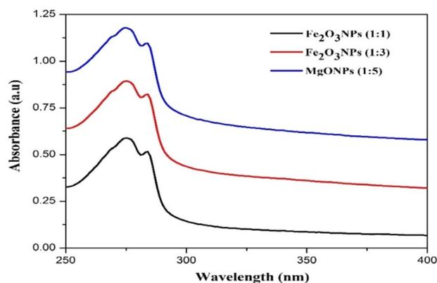
Fig. 5 UV-visible spectrum of Fe<sub>2</sub>O<sub>3</sub>NPs (1 : 1), Fe<sub>2</sub>O<sub>3</sub>NPs (1 : 3), and MgONPs (1 : 5).
