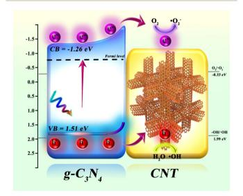
Fig. 8 The schematic of the proposed mechanism of  $g-C_3N_4/CNT$  composites for actual waste drilling filtrate under simulate sun light irradiation.
