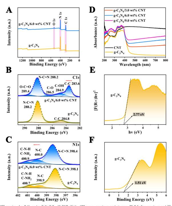
Fig. 4 XPS spectra of  $g-C_3N_4$  and  $g-C_3N_4/6.0$  wt% CNT: (A) the XPS survey spectrum analysis map; (B) C 1s fine spectrum and (C) N 1s fine spectrum; (D) the UV-vis spectra of samples; the bandgap energy diagram of  $g-C_3N_4$  (E) and (F) the valence band (XPS) spectra.
