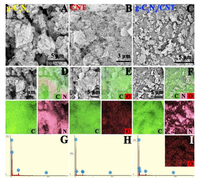
ig. 1 SEM images of (A-C) g-C<sub>3</sub>N<sub>4</sub>, CNT and g-C<sub>3</sub>N<sub>4</sub>/CNT; the corresponding elemental mappings (D-F); and the EDS spectrum (G-I).
