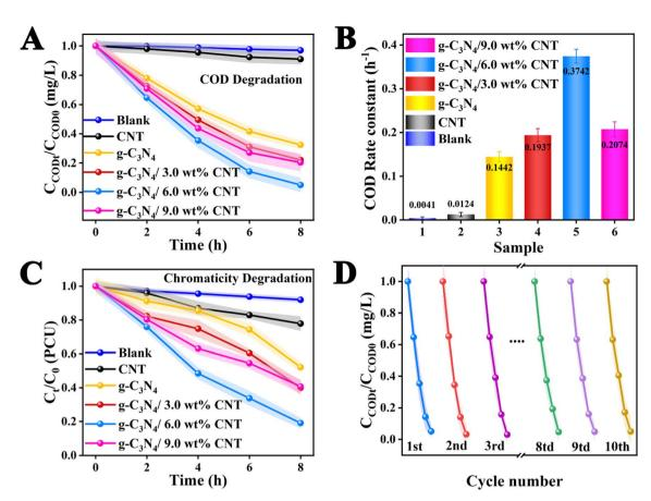
Fig. 5 (A) The COD of the actual waste drilling filtrate photodegradation using each sample during 8 h under simulate sun light irradiation and (B) the corresponding photodegradation rate constants; (C) chromaticity removal rate of actual waste drilling press filtrate and (D) the cyclic tests.
