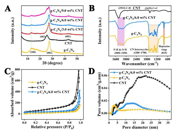
Fig. 3 (A) The XRD patterns of samples; (B) the FTIR spectra of  $g-C_3N_4$ , CNT and  $g-C_3N_4/6.0$  wt% CNT; (C)  $N_2$  adsorption–desorption isotherms and (D) pore volume of samples.
