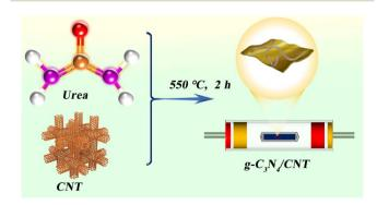
Scheme 1 Synthesis of q-C<sub>3</sub>N<sub>4</sub>/CNT composites.
