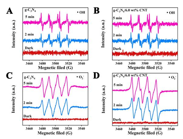
Fig. 7 The ESR spectral analysis of active species \*OH (A and B) and \*O2 (C and B) during photodegradation processes.
