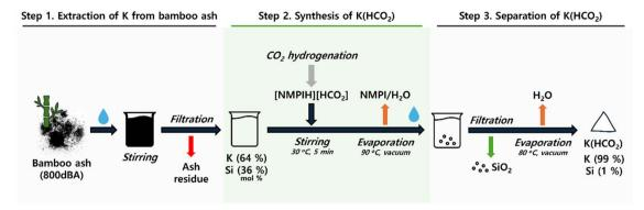
Fig. 4 Production process of K(HCO<sub>2</sub>) from 800dBA and 2.
