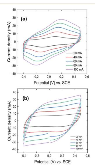
Fig. 3 CV curves of PANI fiber (a), and 3D PANI (b).
