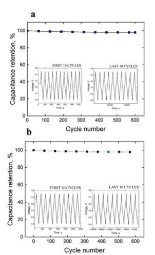
Fig. 4 Cycle life test and GCD curve of the first and last 10 cycles of (a) PANI fiber and (b) 3D crosslinked PANI at a current density of 1 A  $\rm g^{-1}$ .
