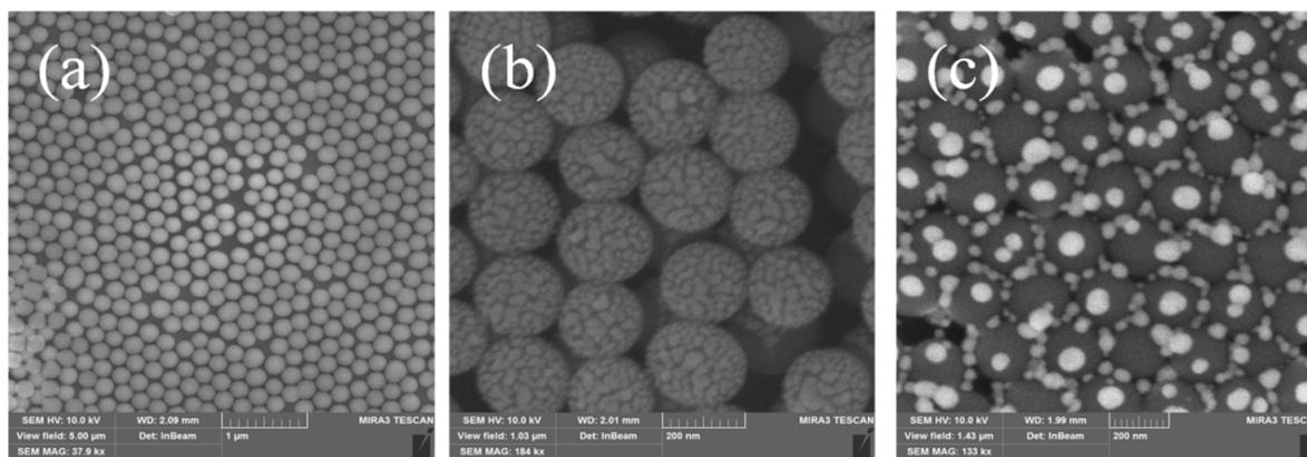
Fig. 2 SEM image of the self-assembled SiO<sub>2</sub> nanospheres on Si substrate (a), spheres covered with 15 nm Ag layer (b), and annealed at 300 °C (c).
