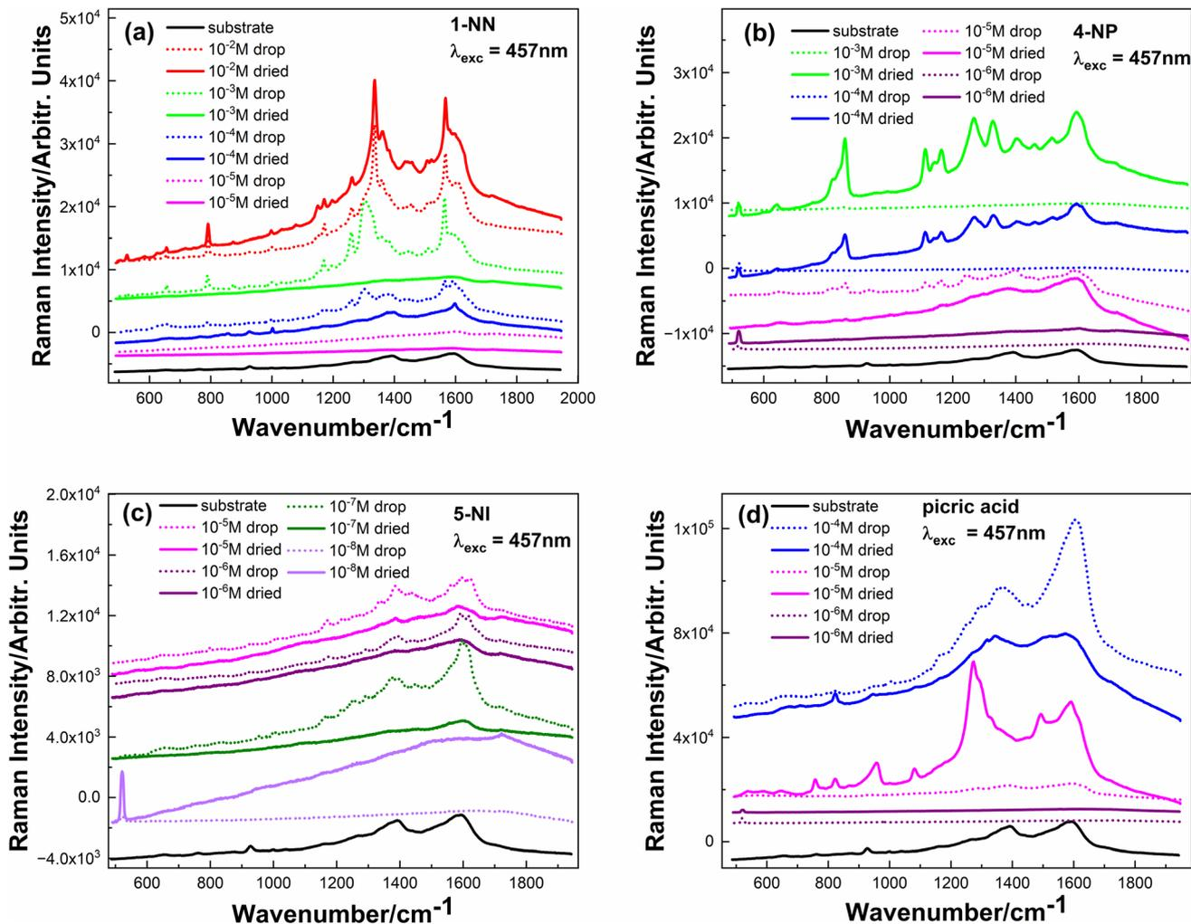
Fig. 5 SERS spectra of samples drop-casted on SiO<sub>2</sub> nanospheres covered with a 15 nm Ag layer: (a) 1-NN, (b) 4-NP, (c) 5-NI, and (d) picric acid. The measurement was performed on the drop of the solution immediately after its deposition (dotted curves) and after the solution was dried (solid curves).
