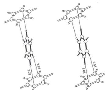
Fig. 2  $\pi$ - $\pi$  stacking between benzene rings.<sup>60</sup>
