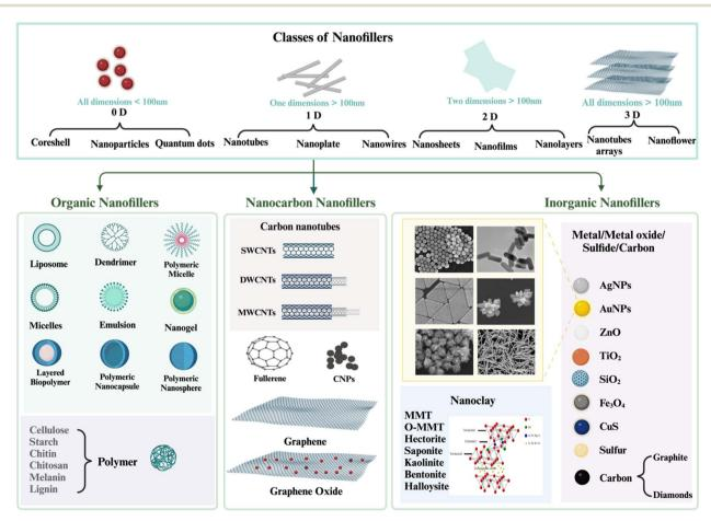
The Schematic and SEM images for different types and shapes of nanofillers. Created with https://www.BioRender.com/.
