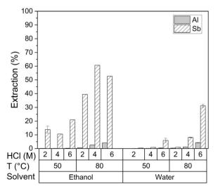
Fig. 1 Leachability of aluminium and antimony at 50  $^{\circ}$ C and 80  $^{\circ}$ C in aqueous and ethanolic HCl solutions of different concentrations at L/S = 10 for 2 h.
