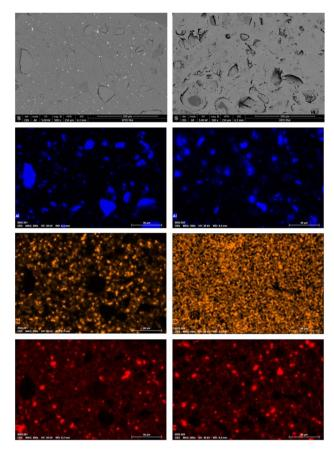
Fig. 5 SEM-EDX photos of (left) untreated PVC material and (right) PVC material leached for 4 h at 80  $^{\circ}$ C in ethanolic 4 M HCl. The top images provide a SEM images, whereas the coloured images below provide EDX images for Al (blue), Sb (yellow) and Si (red). The intense colouring for antimony in the righthand side EDX picture is mainly due to background noise.
