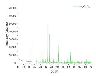
Fig. 4 X-ray diffractogram of the obtained precipitated. All observed diffraction peaks can be assigned to the  $Sb_4Cl_2O_5$  mineral phase.
