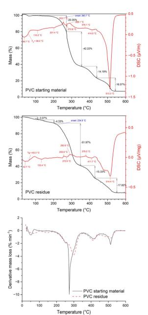
Fig. 2 DSC and TGA curves of the 1 cm  $\times$  1 cm flakes of the original PVC sample (top) and their residue obtained after leaching in 4 M ethanolic HCl solution at 80 °C for 5 h (middle). The derivative mass loss of the two samples is shown in the graph at the bottom.
