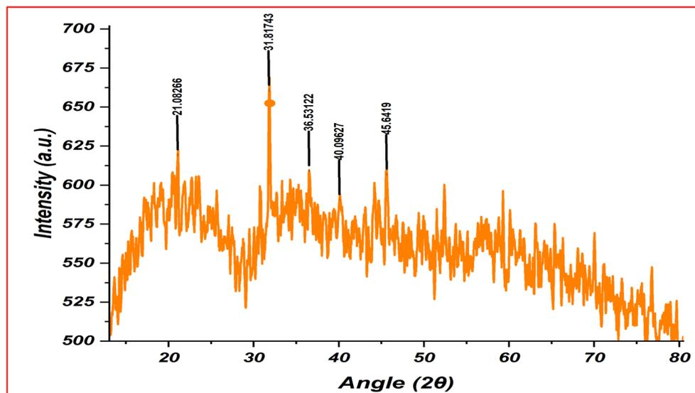
Fig. 8 XRD pattern of synthesized iron oxide nanoparticles.
