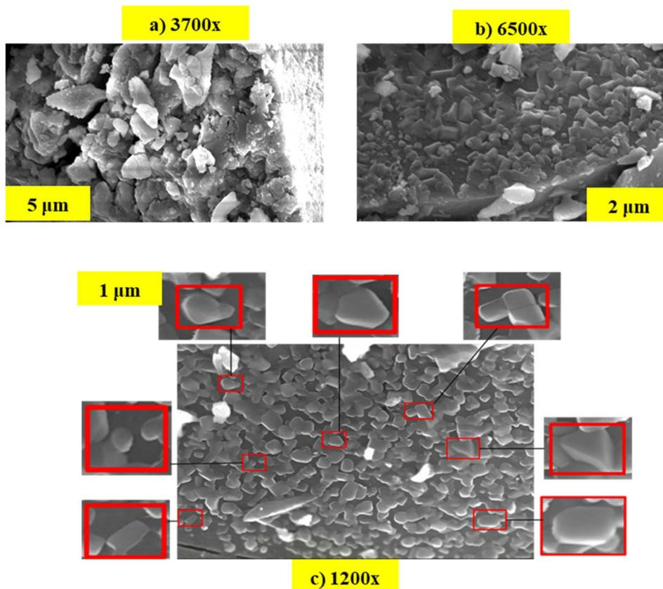
Fig. 5 SEM images of synthesized iron oxide nanoparticles at various magnifications showing detailed morphological differences. (a) Image at 3700 $\times$  magnification, scale bar represents 5  $\mu\text{m}$ . (b) Image at 6500 $\times$  magnification, scale bar represents 2  $\mu\text{m}$ . (c) Image at 1200 $\times$  magnification, scale bar represents 1  $\mu\text{m}$ , highlighting the uniform particle distribution and size variation.
