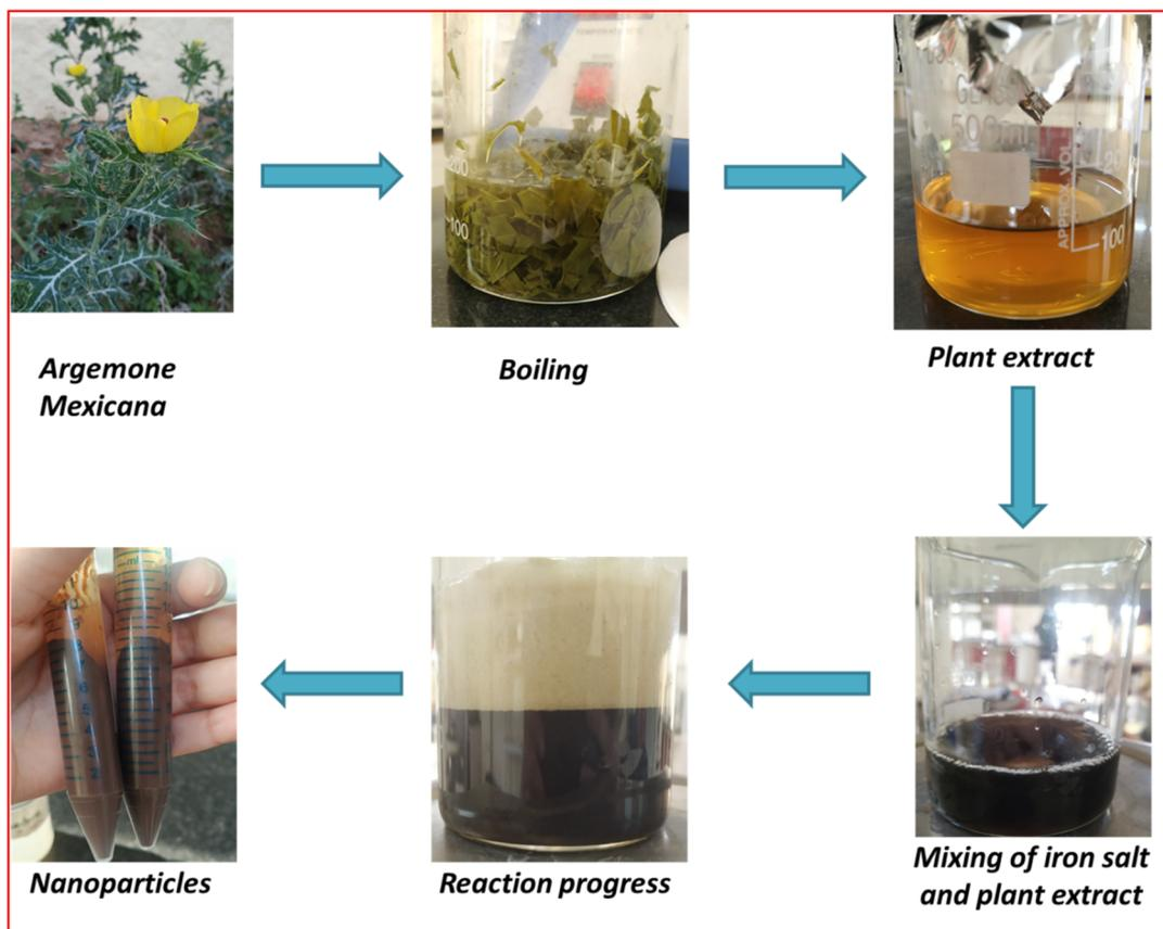
Fig. 2 Green synthesis of iron nanoparticles.
