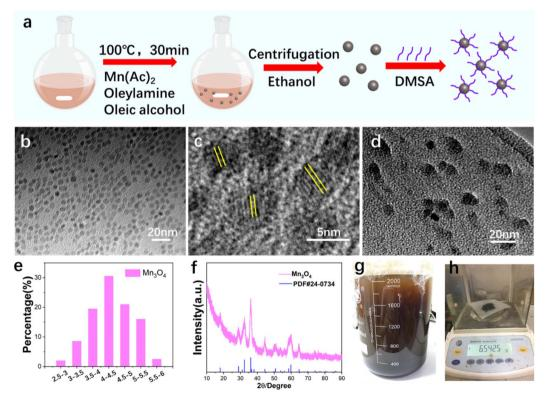
Fig. 1 Synthesis and characterization of ultrasmall  $Mn_3O_4$  nanoparticles. (a) The synthesis scheme of ultrasmall  $Mn_3O_4$  nanoparticles. (b) TEM, (c) HRTEM image of ultrasmall  $Mn_3O_4$  nanoparticles. (d) HRTEM image of  $Mn_3O_4$  nanoparticles. (e) Size distribution statistic and (f) XRD pattern of ultrasmall  $Mn_3O_4$  nanoparticles. (g) Washing procedure and (h) mass production of ultrasmall  $Mn_3O_4$  nanoparticles.
