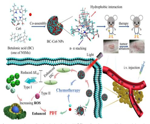
Fig. 10 Schematic of a representative small molecule, betulonic acid (BC)-meditated co-assembled synergistic antitumor BC-Ce6 NP for significantly enhanced chemo-photodynamic combination. Copyright © American Chemical Society, adapted with permission from ref. 44.
