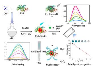
Scheme 1 Schematic illustration of fluorometric/colorimetric dualchannel sensing platform for dopamine detection based on BSA-Cu NPs nanozyme combined with smartphone-assisted analysis.
