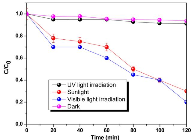
Fig. 11 Plot of  $C/C_0$  versus time via the pristine  $Sb_2S_3$  and Eu-doped  $Sb_2S_3$  films at various doping levels within 120 min at room temperature and atmospheric pressure, under dark conditions and light irradiations.
