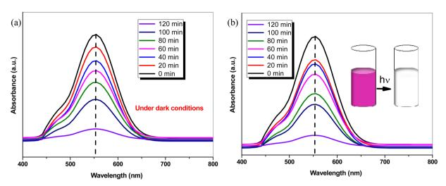
Fig. 13 Temporal evolution of the absorbance spectra of RhB dye solution (a) under dark conditions (b) under visible light irradiation in the presence of 4 at% Eu-doped  $Sb_2S_3$  photocatalyst. The intensity of the absorbance band at 554 nm decreases as the RhB degrades, indicating the photocatalytic activity of the films.
