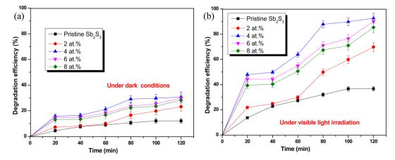
Fig. 12 The photocatalytic degradation efficiency of RhB dye via the pristine Sb<sub>2</sub>S<sub>3</sub> and Eu-doped Sb<sub>2</sub>S<sub>3</sub> photocatalysts at various doping levels within 120 min (a) under dark conditions (b) under visible light irradiation.
