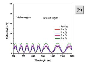
Fig. 8 (a) Spectra of the transmission (T) and (b) reflectivity (R) for pristine and Eu-doped Sb<sub>2</sub>S<sub>3</sub> films at various doping levels, showing the impact of doping on the optical properties of the films.
