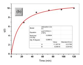
Fig. 14 The adsorption kinetic plots of RhB on 4 at% Eu-doped  $Sb_2S_3$  film fitted with (a) pseudo-first-order, and (b) pseudo-second-order models.
