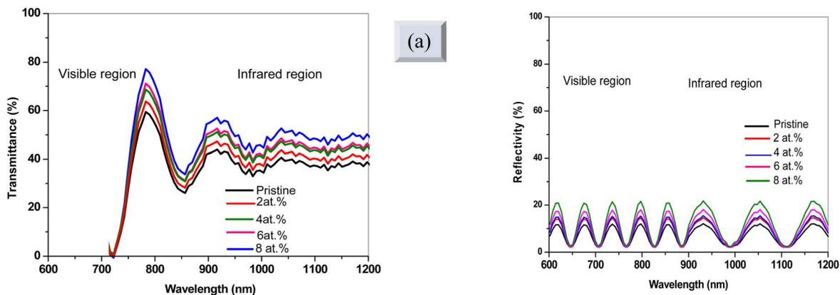
Fig. 8 (a) Spectra of the transmission ( $T$ ) and (b) reflectivity ( $R$ ) for pristine and Eu-doped  $\text{Sb}_2\text{S}_3$  films at various doping levels, showing the impact of doping on the optical properties of the films.
