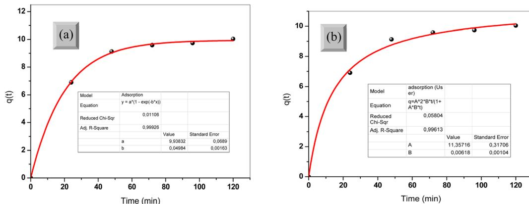
Fig. 14 The adsorption kinetic plots of RhB on 4 at% Eu-doped Sb<sub>2</sub>S<sub>3</sub> film fitted with (a) pseudo-first-order, and (b) pseudo-second-order models.
