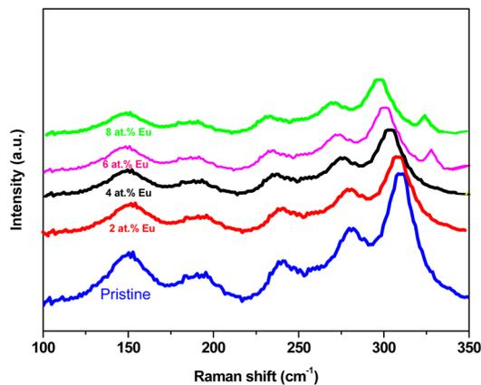
Fig. 3 Raman spectra of pristine and Eu-doped  $\text{Sb}_2\text{S}_3$  films at different doping levels, illustrating the effects of Eu doping on the vibrational modes of the  $\text{Sb}_2\text{S}_3$  thin films.
