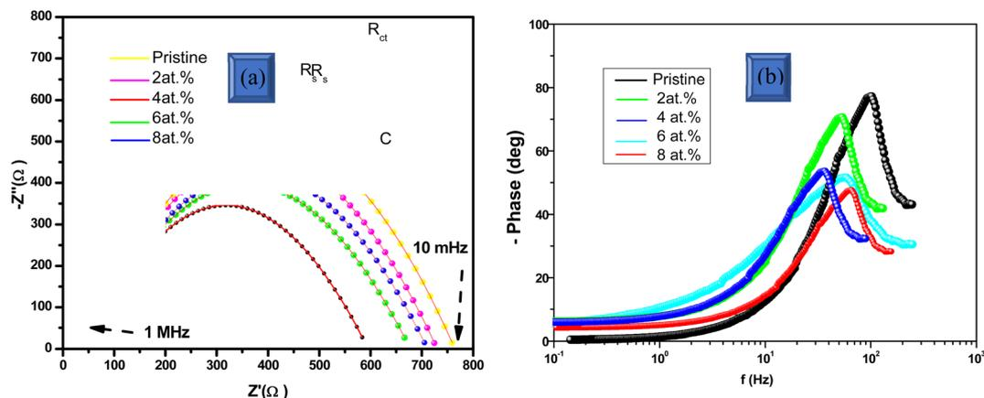
Fig. 10 (a) Electrochemical impedance spectra of pristine and Eu-doped  $\text{Sb}_2\text{S}_3$ . Solid and dashed lines represent the experimental and fitted data, respectively. Inset (a) shows the representation of the Randles equivalent circuit model. (b) Bode phase angle plots for all samples.
