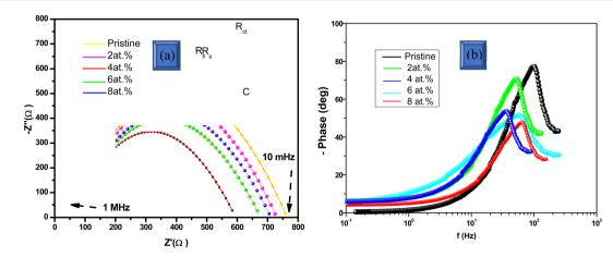
Fig. 10 (a) Electrochemical impedance spectra of pristine and Eu-doped  $Sb_2S_3$ . Solid and dashed lines represent the experimental and fitted data, respectively. Inset (a) shows the representation of the Randles equivalent circuit model. (b) Bode phase angle plots for all samples.
