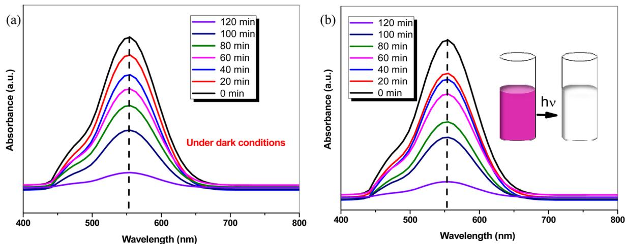
Fig. 13 Temporal evolution of the absorbance spectra of RhB dye solution (a) under dark conditions (b) under visible light irradiation in the presence of 4 at% Eu-doped  $\text{Sb}_2\text{S}_3$  photocatalyst. The intensity of the absorbance band at 554 nm decreases as the RhB degrades, indicating the photocatalytic activity of the films.
