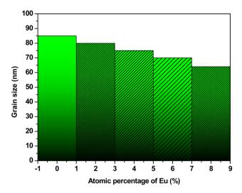
Fig. 6 The evolution of the grain size of  $Sb_2S_3$  thin films as a function of Eu content.
