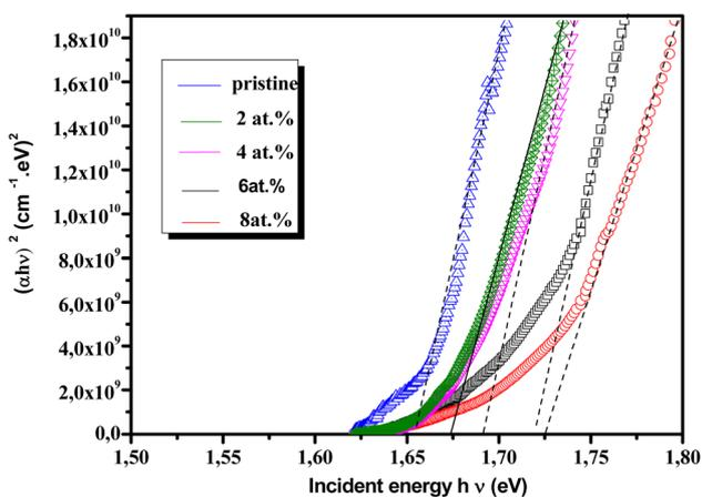
Fig. 9 The optical bandgap of pristine and Eu-doped  $\text{Sb}_2\text{S}_3$  at various doping levels were analyzed using a Tauc plot derived from the optical transmittance and reflectivity spectra of the glass/ $\text{Sb}_2\text{S}_3$  layer stack.
