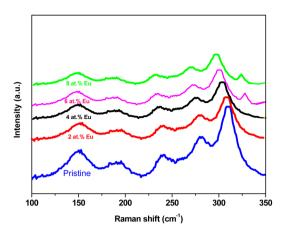
Fig. 3 Raman spectra of pristine and Eu-doped  $\mathrm{Sb}_2\mathrm{S}_3$  films at different doping levels, illustrating the effects of Eu doping on the vibrational modes of the  $\mathrm{Sb}_2\mathrm{S}_3$  thin films.
