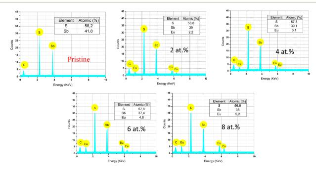
Fig. 7 EDS spectra of  $Sb_2S_3$  thin films, thermally annealed at 300 °C for 5 minutes and doped with varying Eu content, illustrating the elemental composition and the influence of Eu doping on the material's chemical structure.
