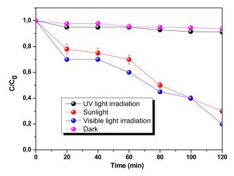
Fig. 11 Plot of  $C/C_0$  versus time via the pristine  $Sb_2S_3$  and Eu-doped Sb<sub>2</sub>S<sub>3</sub> films at various doping levels within 120 min at room temperature and atmospheric pressure, under dark conditions and light irradiations
