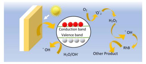
Fig. 16 The mechanism of the Eu-doped  $Sb_2S_3$  (4 at%) photocatalyst activity toward RhB dye under visible light irradiation.
