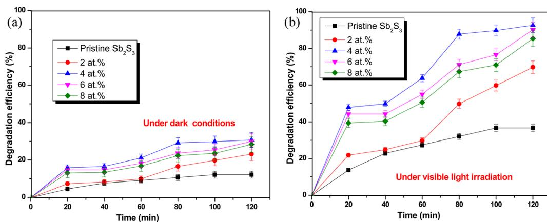
Fig. 12 The photocatalytic degradation efficiency of RhB dye via the pristine  $Sb_2S_3$  and Eu-doped  $Sb_2S_3$  photocatalysts at various doping levels within 120 min (a) under dark conditions (b) under visible light irradiation.
