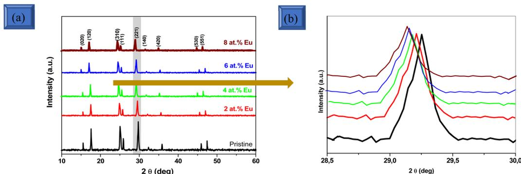
Fig. 1 (a) GIXRD patterns of pristine and Eu-doped  $\text{Sb}_2\text{S}_3$  films at various doping levels. (b) A zoomed-in view of the (221) peak in the  $2\theta$  range of  $28.5\text{--}30^\circ$  for both pristine and Eu-doped  $\text{Sb}_2\text{S}_3$  films, showing the impact of doping on the main peak position.
