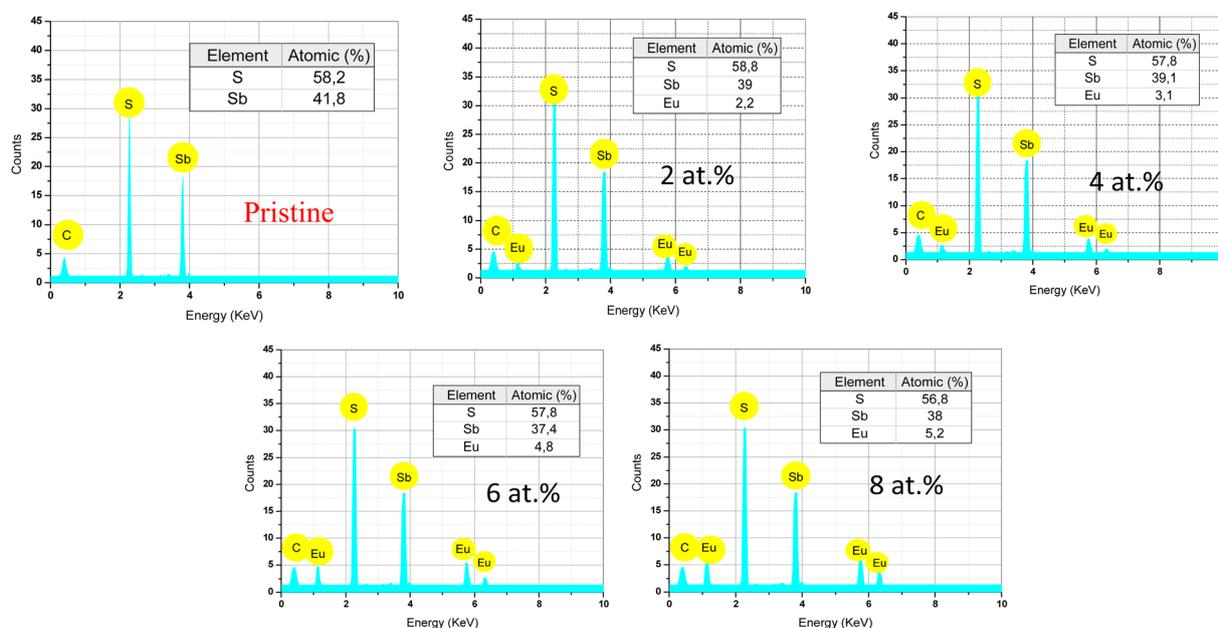
Fig. 7 EDS spectra of  $\text{Sb}_2\text{S}_3$  thin films, thermally annealed at 300 °C for 5 minutes and doped with varying Eu content, illustrating the elemental composition and the influence of Eu doping on the material's chemical structure.
