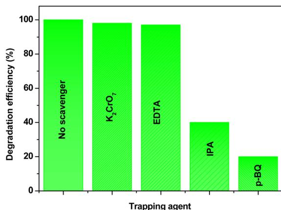
Fig. 15 Radical scavenger study for active species during the photo-degradation of RhB wastewater employing Eu-doped Sb<sub>2</sub>S<sub>3</sub> (4 at%) photocatalyst under visible light.
