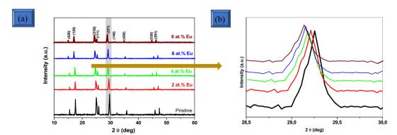
Fig. 1 (a) GIXRD patterns of pristine and Eu-doped Sb<sub>2</sub>S<sub>3</sub> films at various doping levels. (b) A zoomed-in view of the (221) peak in the  $2\theta$  range of 28.5–30° for both pristine and Eu-doped Sb<sub>2</sub>S<sub>3</sub> films, showing the impact of doping on the main peak position.
