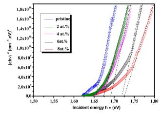
Fig. 9 The optical bandgap of pristine and Eu-doped  $Sb_2S_3$  at various doping levels were analyzed using a Tauc plot derived from the optical transmittance and reflectivity spectra of the glass/ $Sb_2S_3$  layer stack.
