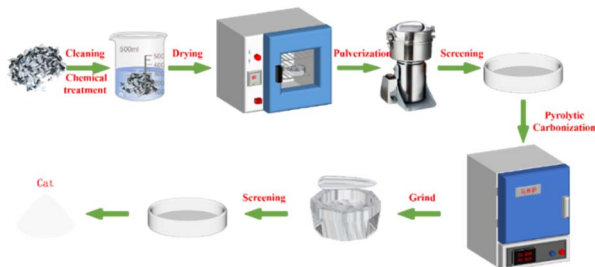
Fig. 1 Schematic diagram of sunflower seed shell matrix catalyst preparation.
