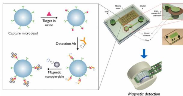
**Fig. 9** The schematics of the  $\mu$ UNPD assay for CysC detection. Firstly, capture antibody conjugated microbeads, followed by TCO conjugated detection antibodies, and finally amino modified magnetic nanoparticles, are added for the CysC detection from the urine sample on the microchip. Reprinted with permission from ref. 95. Copyright: © 2015 Chung *et al.*
