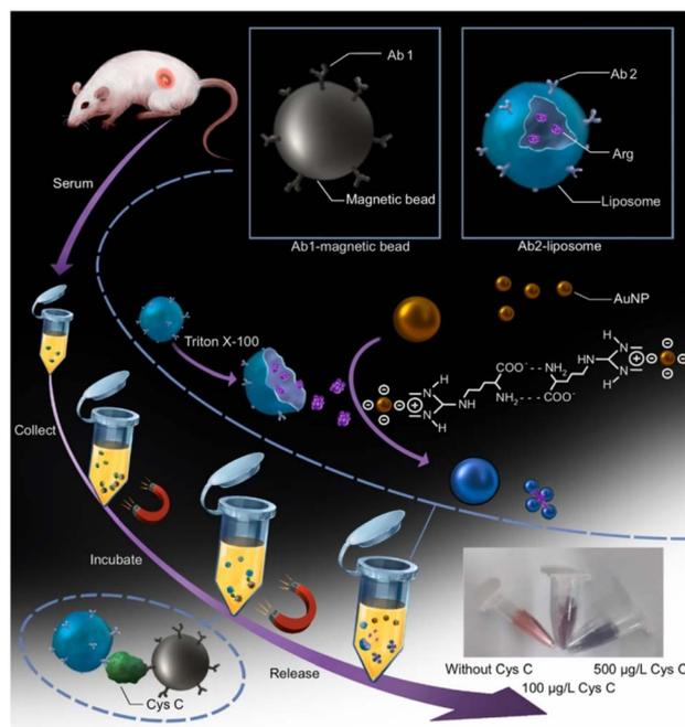
Fig. 6 Schematic illustration of the principle and operation steps of CysC sensor made by a arginine liposome-amplified colorimetric immunoassay. Reprinted with permission from.<sup>80</sup> Copyright © 2022 Elsevier B.V.
