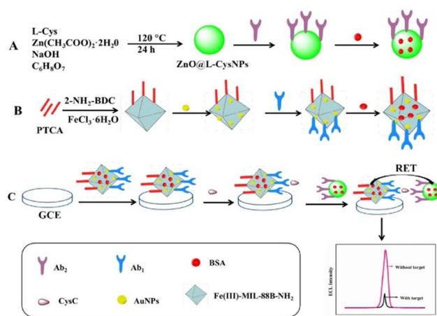
Fig. 8 (A) Schematic showing the preparation of  $\text{ZnO@L-CysNPs/Ab2}$  (A) and synthesis of  $\text{PTCA@Fe(III)-MIL-88B-NH}_2\text{@Au/Ab1}$ . (B) The preparation of ECL-FRET immunosensor as well as (C) the detection of CysC. Reprinted with permission from ref. 93. Copyright © 2023 Elsevier B.V.
