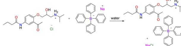
Scheme 1 Synthesis of the Acebutolol-tetraphenyl borate ion-pair complex.
