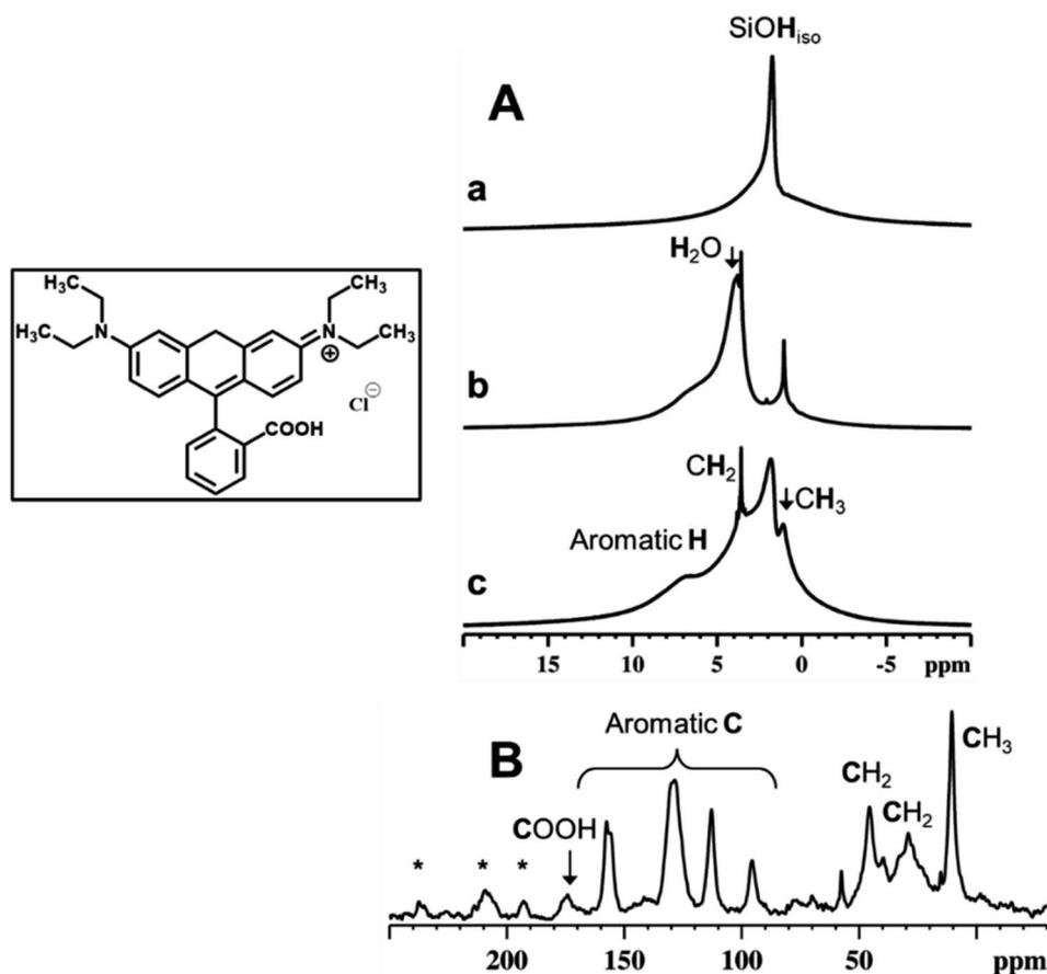
Fig. 7 <sup>1</sup>H MAS NMR (A) spectra of RH-nanoMCM after dehydration (a) and of RH-nanoMCM + RhB before (b) and after (c) dehydration. <sup>13</sup>C CPMAS NMR (B) spectrum of RH-nanoMCM + RhB. Inset shows the molecular structure of RhB. \* spinning sidebands.
