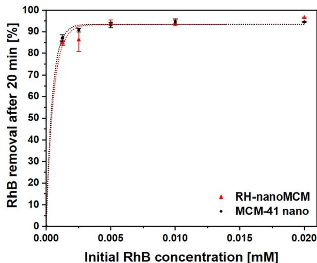
Fig. 6 Rhodamine B removal percentages after a contact time of 20 min with RH-nanoMCM (triangles) and MCM-41 nano (circles). The initial RhB concentrations are  $2.0 \times 10^{-2}$ ,  $1.0 \times 10^{-2}$ ,  $5.0 \times 10^{-3}$ ,  $2.5 \times 10^{-3}$  and  $1.2 \times 10^{-3}$  mmol L<sup>-1</sup>. The error bars represent the standard deviations over three measurements.
