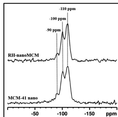
Fig. 4 <sup>29</sup>Si MAS NMR spectra of RH-nanoMCM and MCM-41 nano.
