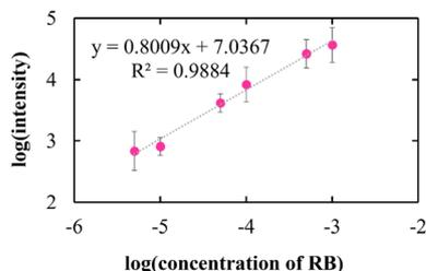
Fig. 9 The log–log plot of the peak intensity of RhB at 1643 cm<sup>-1</sup>.
