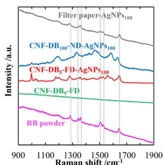
**Fig. 6** Raman spectra of RhB deposited on the filter paper-AgNPs<sub>100</sub>, CNF-DB<sub>100</sub>-ND-AgNPs<sub>100</sub>, CNF-DB<sub>5</sub>-FD-AgNPs<sub>100</sub> and CNF-DB<sub>5</sub>-FD. The samples were prepared by reduction with NaBH<sub>4</sub>. The dotted lines indicate the peak positions of RhB.
