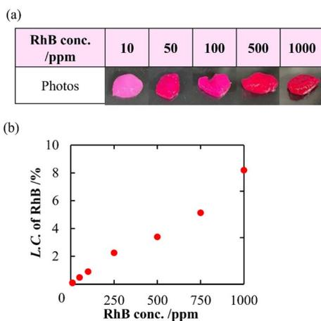
Fig. 4 Photo images of CNF-DB<sub>5</sub>-FD after loading of RhB (a) and change in the loading capacity of RhB into CNF-DB<sub>5</sub>-FD with RhB concentration (b).
