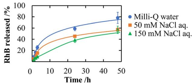
Fig. 5 Release profiles of RhB from CNF-DB<sub>5</sub>-FD at different ionic strengths.
