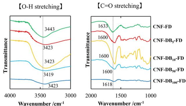
Fig. 1 FT-IR spectra of C=O stretching band (right) and O-H stretching band (left) for lyophilized CNF (CNF-FD) and CNF-DB<sub>x</sub>-FD. The numbers indicate the wavenumber corresponding to each vibration mode.
