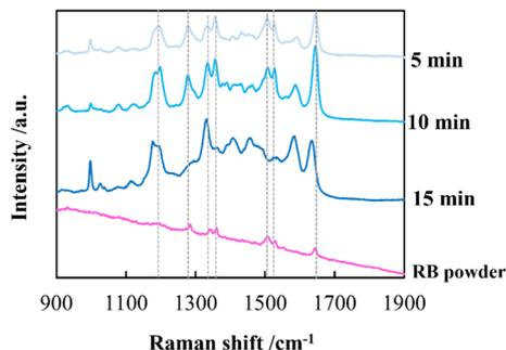
Fig. 7 Raman spectra of RhB deposited on CNF-DB<sub>5</sub>-FD-Ag<sub>100</sub>. The samples were prepared by reduction with sodium citrate under microwave irradiation for different periods. The dotted lines indicate the peak positions of RhB.
