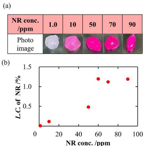
Fig. 3 Photo images of CNF-DB<sub>5</sub>-FD after loading of NR (a) and change in the loading capacity of NR into CNF-DB<sub>5</sub>-FD with NR concentration (b).
