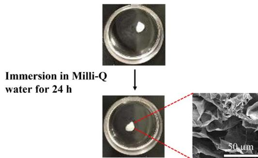
Fig. 2 Photo images showing the structural stability of CNF-DB<sub>5</sub>-FD in Milli-Q water. The inset shows its cross-sectional SEM image 24 h after immersion in Milli-Q water.
