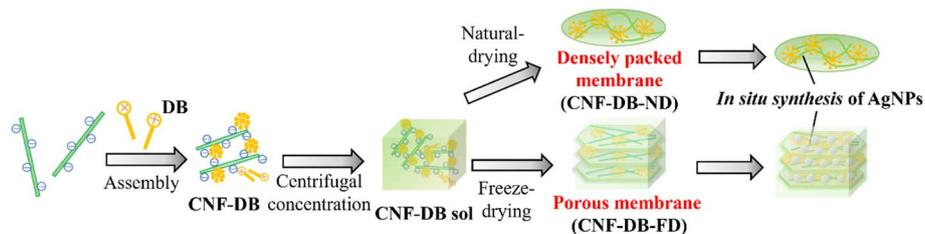
**Scheme 1** Schematic illustration for preparation of a CNF densely packed membrane and a CNF porous membrane *via* surfactant-induced assembly. *In situ* reduction of Ag ions was conducted to prepare an AgNPs-CNF composite membrane (*in situ* synthesis of AgNPs).
