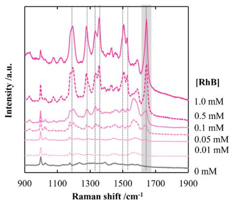
Fig. 8 Raman spectra of RhB deposited on CNF-DB<sub>5</sub>-FD-AgNPs<sub>100</sub> at different RhB concentrations. CNF-DB<sub>5</sub>-FD-AgNPs<sub>100</sub> was prepared by reduction with sodium citrate under microwave irradiation for 10 min.
