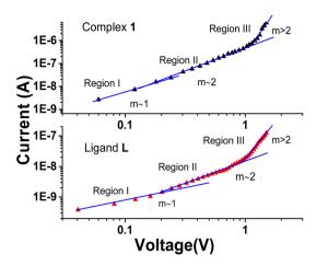
Fig. 6 Logarithmic plot of I-V characteristics of Al/complex 1/ITO and Al/ligand L/ITO structured device.
