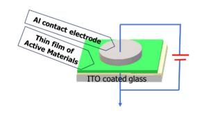
**Scheme 1** Schematic of metal-semiconductor junction for electrical measurements.
