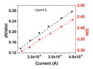
Fig. 7 (a)  $dV/d \ln I$  vs. I and H(I)vs. I graphs for complex 1. (b)  $dV/d \ln I$  vs. I and H(I)vs. I graphs for ligand L.
