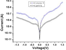
Fig. 5 I-V characteristics of Al/complex 1/ITO and Al/ligand L/ITO (for better clarity it is also shown in inset) in (top) linear scale and (bottom) in semi-log scale.
