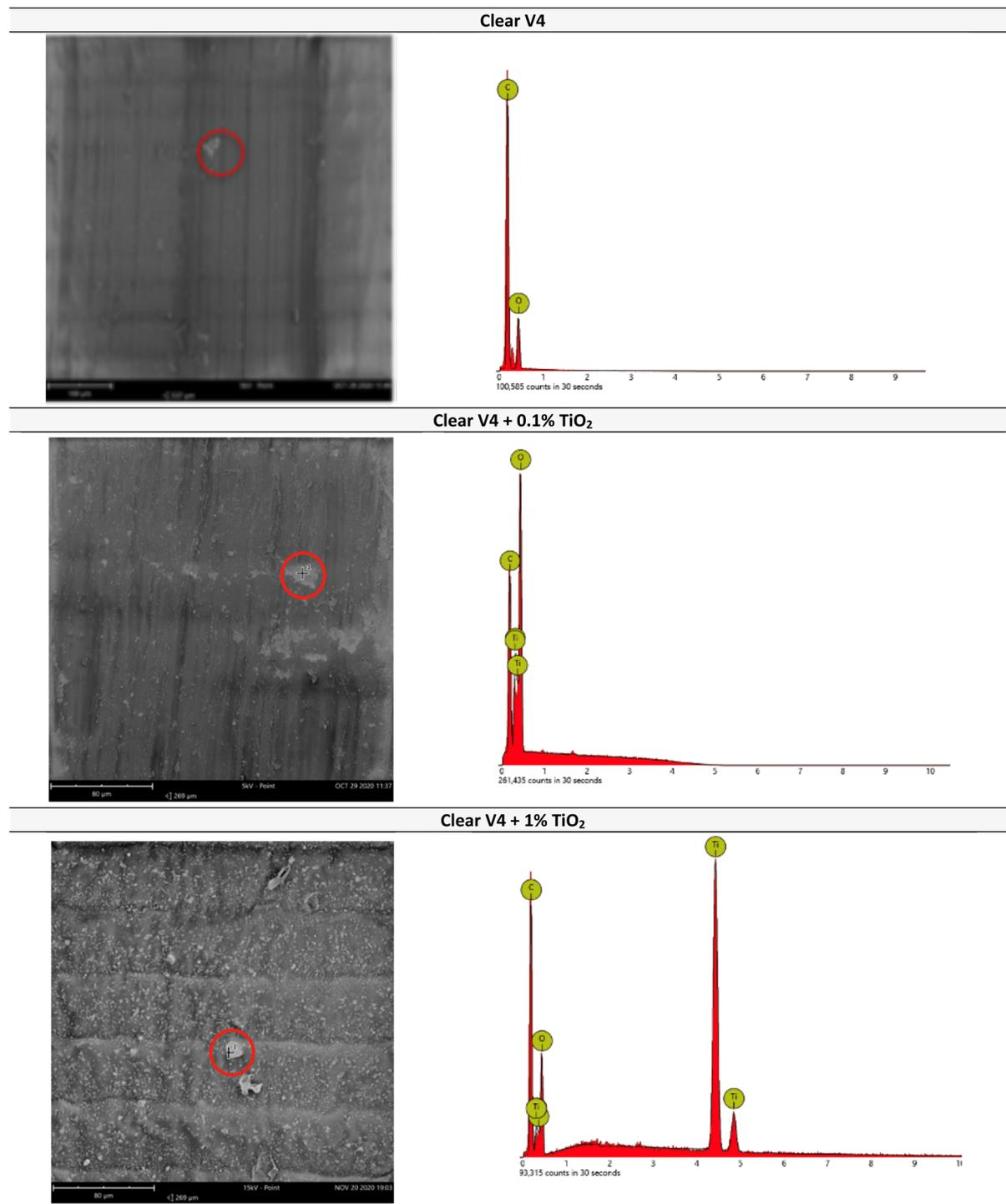
Fig. 6 SEM images and EDS spectrum (taken from the highlighted zones) for plane plate printed at 0° for each material: Clear V4, Clear V4 + 0.1% TiO<sub>2</sub> and Clear V4 + 1% TiO<sub>2</sub>.
