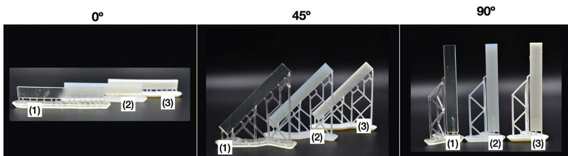
Fig. 9 Photographs for materials printed at different printing angles, these plane plates were used for the DMA test. Legend: (1) Clear V4, (2) Clear V4 + 0.1%  $\text{TiO}_2$  and (3) Clear V4 + 1%  $\text{TiO}_2$ .
