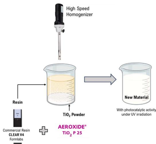
Fig. 1 Dispersion process of TiO<sub>2</sub> powder on Clear V4 commercial resin.
