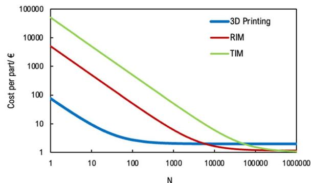
Fig. 14 Comparison of costs per part for plastic manufacturing techniques (3D printing, RIM and TIM) on a logarithmic scale.
