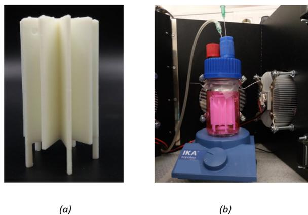
Fig. 12 (a) 3D printed structure and (b) experimental setup of photocatalytic degradation of Rh<sub>B</sub>. ( $T = 20\text{ }^{\circ}\text{C}$ ;  $[\text{Rh}_B]_{\text{in}} = 10\text{ }\mu\text{M}$ ;  $\lambda_{\text{max}} = 370\text{ nm}$ ; total irradiance  $\approx 520\text{ W m}^{-2}$ ).
