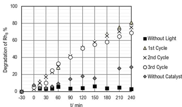
Fig. 13 Photocatalytic degradation of Rh<sub>B</sub> over 3 consecutive cycles.
