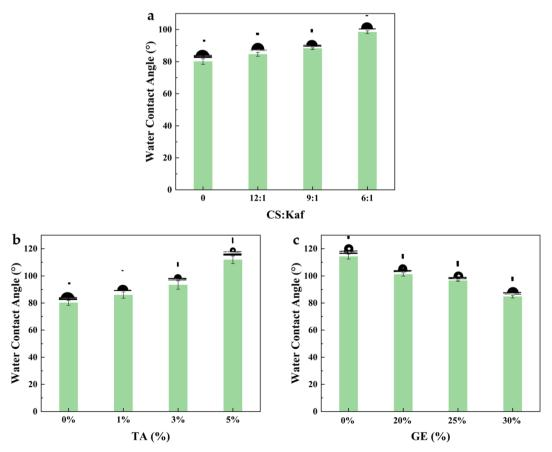
Water contact angles of composite films with different CS contents: Kaf (a), TA (b), and GE (c) contents
