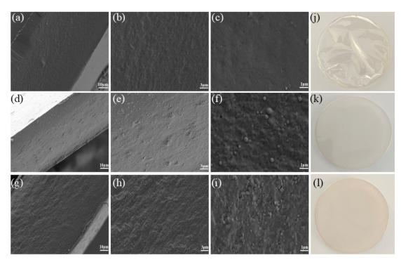
Fig. 2 SEM and optical electron microscopy image images of composite film sections: (a-c and j) CS film; (d-f and k) C9K1G20 composite film; (q-i and I) C9K1T5G20 composite film
