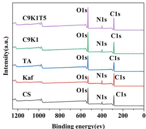
Fig. 10 Full XPS spectra of the composite film.
