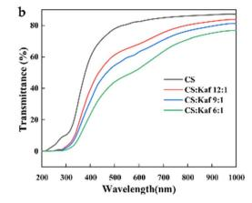
Fig. 8 Transmittance of composite films with different TA (a) and CS: Kaf (b) contents.
