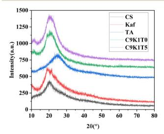
Fig. 9 XRD patterns of different concentrations of TA.
