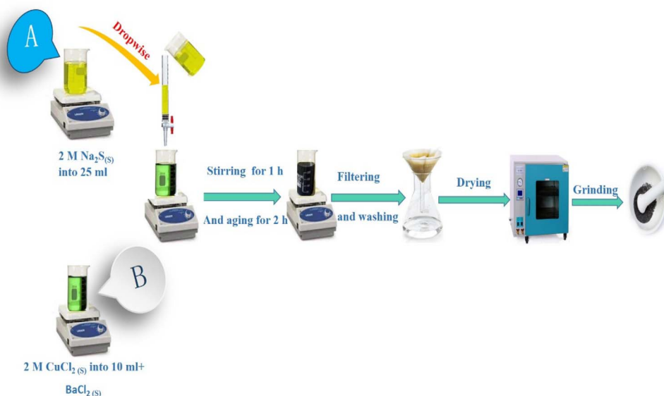
Fig. 1 Schematic diagram of the steps used for the synthesis of pure and Ba-doped CuS nanoparticles.
