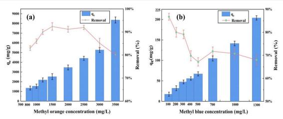
Fig. 4 Effects of the initial concentration of single-component dyes on the adsorption capacity of Zn/Co-ZIF@CNTs: (a) MO and (b) MB.
