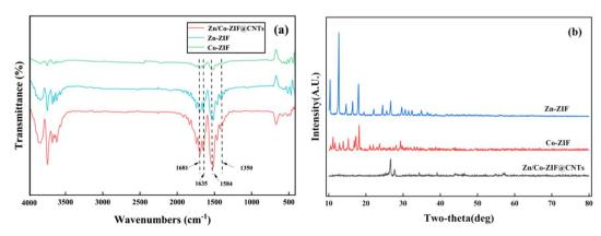
Fig. 3 (a) FT-IR spectra for Zn/Co-ZIF@CNTs and Co-ZIF and Zn-ZIF. (b) XRD patterns for Zn/Co-ZIF@CNTs and Co-ZIF and Zn-ZIF.
