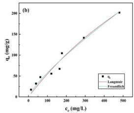
Fig. 9 Adsorption of (a) MO and (b) MB by Zn/Co-ZIF@CNTs. The Langmuir and Freundlich adsorption isotherm models were compared.
