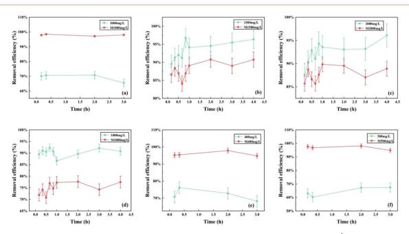
Fig. 5 Removal rate of Zn/Co-ZlF@CNTs for different mixed concentrations of MO and MB: (a) MO 1000 mg  $L^{-1}$ , (b) MO 1500 mg  $L^{-1}$ , (c) MO 2000 mg  $L^{-1}$ , (d) MB 400 mg  $L^{-1}$ , (e) MB 500 mg  $L^{-1}$ , and (f) MB 1000 mg  $L^{-1}$ .
