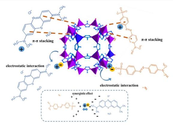
Fig. 10 The possible adsorption mechanism of Zn/Co-ZIF@CNTs for MO and MB.
