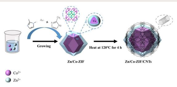
Fig. 1 The synthetic schematic diagram for preparing Zn/Co-ZIF@CNTs
