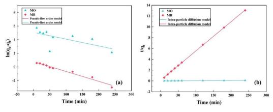
Fig. 8 The adsorption kinetics of MO and MB: (a) pseudo-first order kinetic and (b) pseudo-second-order kinetic.
