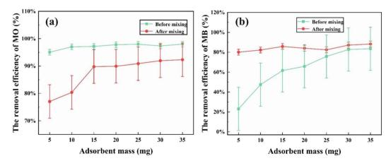
Fig. 7 Removal rate of Zn/Co-ZIF@CNTs for different sorbent content; (a) MO and (b) MB.
