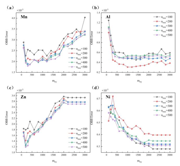
Fig. 4 The influence of different parameters ( $n_{\text{tree}}$  and  $m_{\text{try}}$ ) on OOB Error in RFR model.
