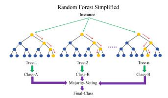
Fig. 2 The schematic diagram of the random forest principle
