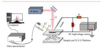
Fig. 1 Schematic diagram of fs-LA-SIBS.
