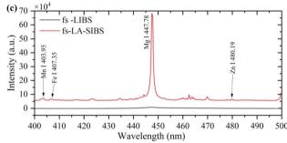
Fig. 3 (a) Shows the plasma emission spectra of different magnesium alloy samples at wavelengths from 300 to 500 nm; comparing the plasma spectra recorded in fs-LA-SIBS and fs-LIBS, (b) 300-400 nm and (c) 400-500 nm.
