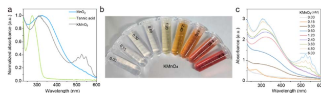
Fig. 1 (a) Normalized UV-vis spectra of MnO 2 , tannic acid and KMnO 4 . (b) Digital photograph and (c) UV-vis spectra of the mixture with different concentration of KMnO 4 ranging from 0 to 6.0 mM.
