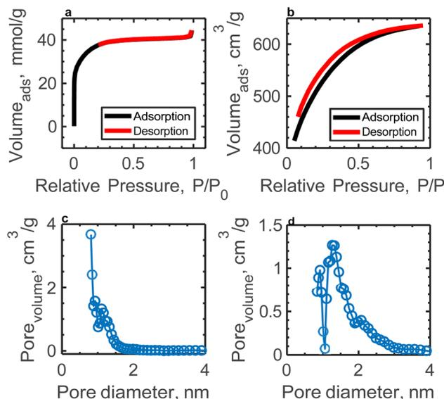
Fig. 1 Pore structure analysis of AC and AC-10BRGO (a) N<sub>2</sub> adsorption-desorption isotherms of AC, (b) N<sub>2</sub> adsorption-desorption isotherms of AC-10BRGO, (c) pore size distribution of AC, and (d) pore size distribution of AC-10BRGO.
