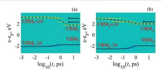
Fig. 6 Supercell calculated charge carrier dynamics for states in (a)  $\Gamma$ - and (b) Z-points in Brillouin zone. The arrows show the intermediate states where excitation is temporarily delayed during the relaxation process.
