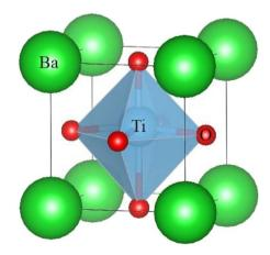
Fig. 1 Crystal structure of tetragonal BaTiO<sub>3</sub>
