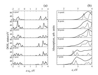
Fig. 3 (a) DOS (b) absorption static (dotted lines) and at  $T=300~{\rm K}$  (solid lines) calculated at different k-points.
