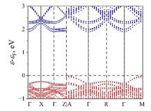
Fig. 2 Element-projected band structure of  $BaTiO_3$  supercell. Red and blue symbols correspond to O and Ti atoms, respectively.
