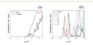
Fig. 4 (a) PBE + U calculated total linear absorption spectra for static BaTiO $_3$  lattice and at T=300 K. (b) HSE06 calculated linear absorption spectra for static BaTiO $_3$  lattice: total absorption and contribution of each irreducible k-point.
