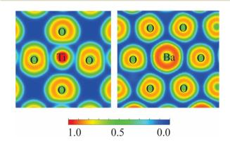
Fig. 9 Projection of ELF on planes passing through Ti–O (left panel) and Ba–O (right panel) bonds in the lattice of  $BaTiO_3$ . Color code blue (ELF = 0) and red (ELF = 1.0) represents full absence and full presence of electron pair in actual point of space.
