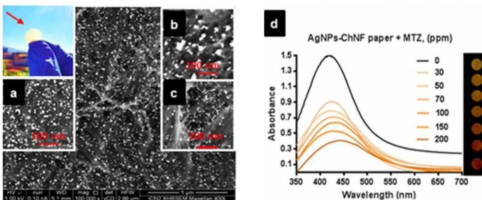
Fig. 24 Scanning electron micrographs of the fabricated AgNPs-ChNF paper: (a) *in situ* synthesized AgNPs-ChNF; (b) AgNPs-ChNF in the presence of 100 ppm MTZ; (c) AgNPs-ChNF paper in the presence of 3 ppm  $\text{CN}^-$ . The inset image (upper left) shows a digital photograph of the fabricated AgNPs-ChNF paper, and (d) displays the AgNPs-ChNF paper upon the addition of MTZ (0–200 ppm).<sup>112</sup>
