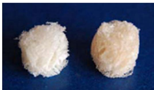
Fig. 20 Chitin scaffold (left) and chitin/nano Ag composite scaffold (right) are suitable for wound healing applications.<sup>180</sup>
