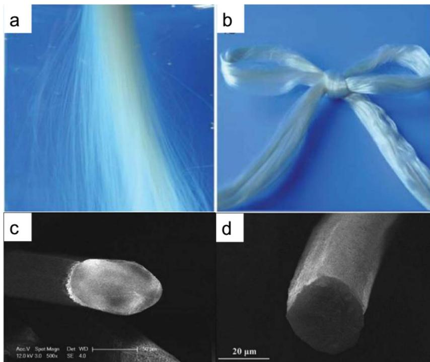
Fig. 7 Photograph of (a) freshly spun chitin fibers in water and (b) air-dried fibers. SEM images of the chitin fibers (c) lyophilized and fractured in liquid nitrogen and (d) air-dried.<sup>44</sup>
