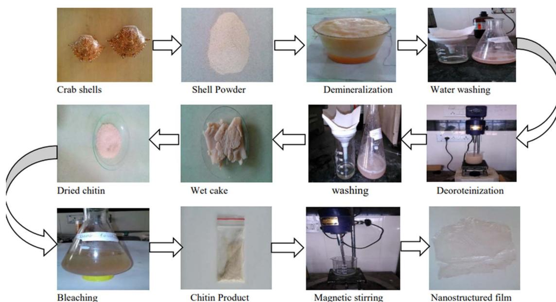
Fig. 25 Photographic presentation of nanostructured film production from crab shells.<sup>59</sup>
