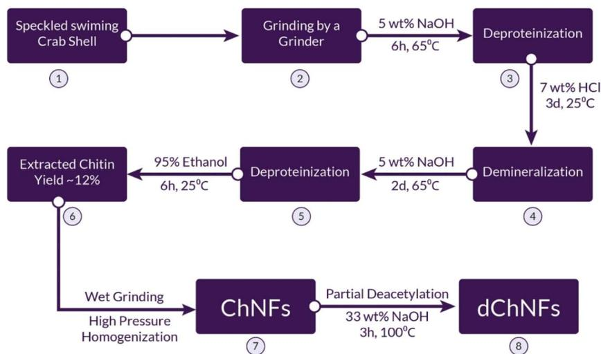
Fig. 12 Schematic illustration of the preparation of ChNFs and dChNFs from speckled swimming crab shells.<sup>24</sup>
