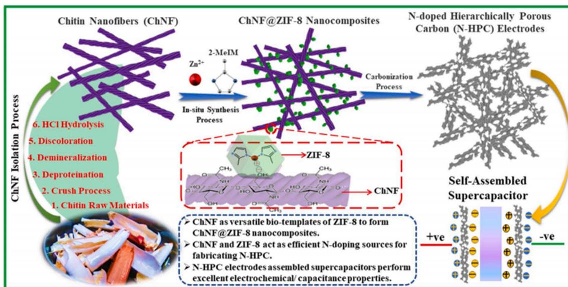
Fig. 27 Schematic illustration of the preparation of N-doped hierarchically porous carbon electrodes for high-performance supercapacitors.<sup>227</sup>
