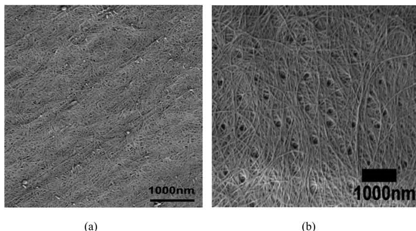
Fig. 13 (a) FE-SEM micrograph of ChNFs from black tiger prawn shells; (b) FE-SEM micrograph of the surface of the black tiger prawn shell after removing the matrices.<sup>28</sup>
