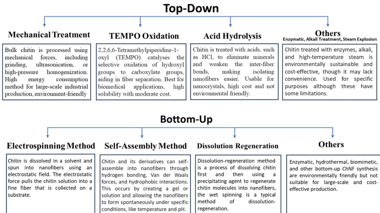
Fig. 9 The various top-down and bottom-up approaches for ChNF synthesis.<sup>36</sup>
