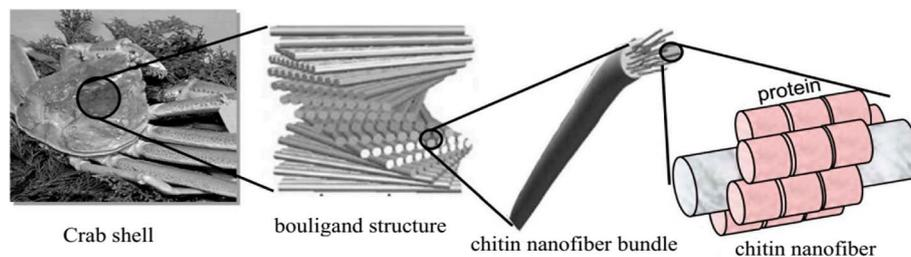
Fig. 10 Schematic presentation of the exoskeleton structure of crab shells.<sup>1</sup>
