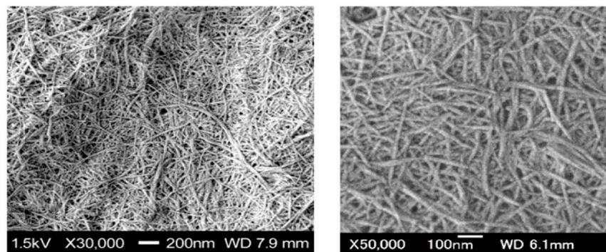
Fig. 11 SEM images of ChNFs from crab shell after grinder treatment.<sup>1</sup>
