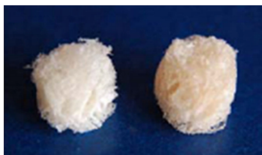
Fig. 20 Chitin scaffold (left) and chitin/nano Ag composite scaffold (right) are suitable for wound healing applications. 180
