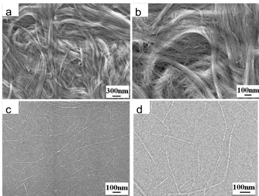
Fig. 4 (a and c) SEM images of the cationized chitin and homogenized chitin with a pH of 4.1, respectively; (b and d) SEM images with higher magnification in comparison to (a) and (c), respectively.<sup>30</sup>
