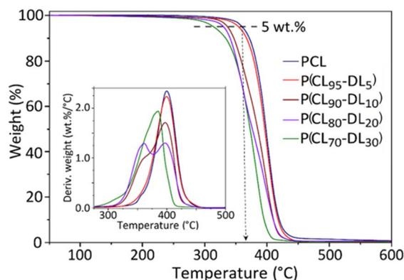
Fig. 6 TGA traces of PCL and P(CL-DL) copolymers.
