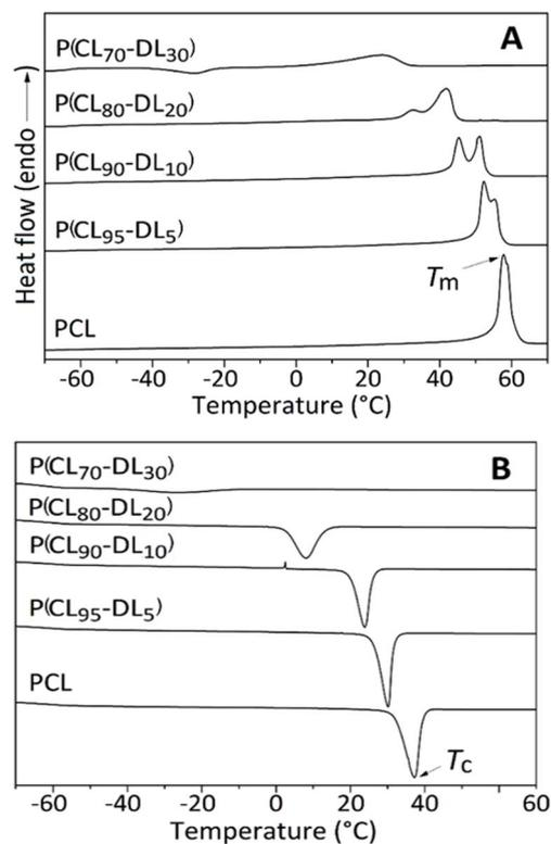
Fig. 7 Heating (A) and cooling (B) DSC traces of the PCL and P(CL–DL) copolymers.
