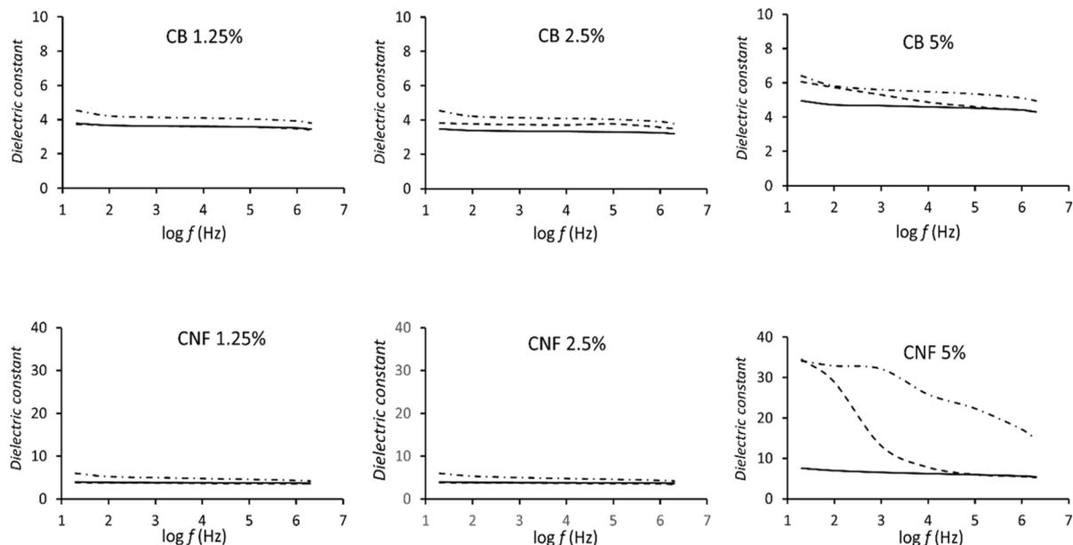
Fig. 11 Dielectric constant – frequency plots of composites of the series I (solid lines), series II (dash lines) and series III (dash-dot lines).
