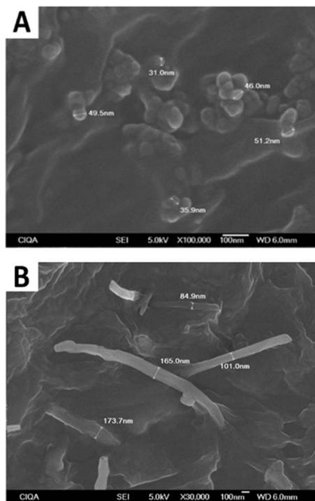
Fig. 10 SEM micrographs of P(CL<sub>90</sub>-DL<sub>10</sub>)/CB<sub>5</sub> (A) and P(CL<sub>90</sub>-DL<sub>10</sub>)/CNF<sub>5</sub> (B).
