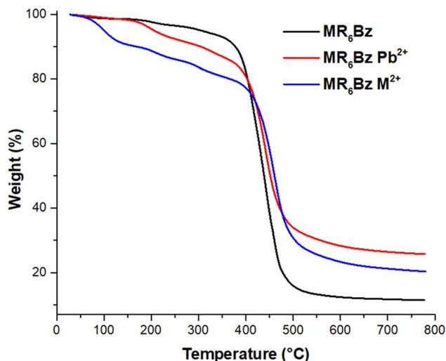
Fig. 13 Thermograms of pristine MR<sub>6</sub>Bz resin (black), Pb<sup>2+</sup>-loaded MR<sub>6</sub>Bz (red) and M<sup>2+</sup>-loaded MR<sub>6</sub>Bz (blue) obtained under a N<sub>2</sub> atmosphere. M<sup>2+</sup> denotes a mixture of divalent cations.
