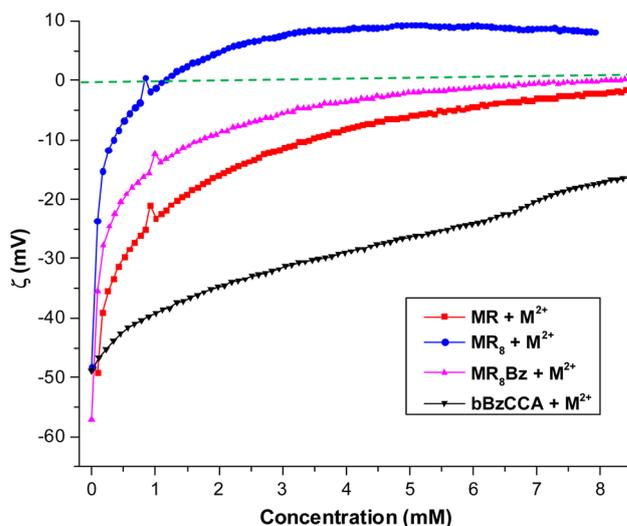
Fig. 8  $\zeta = f[M^{n+}]$  profiles of bBzCCA, MR, MR<sub>8</sub> and MR<sub>8</sub>Bz obtained by titration with a mixture of metal ions. Mass of resin: 20 mg. Volume: 20 mL. Solvent: deionized water. pH: 5.0.
