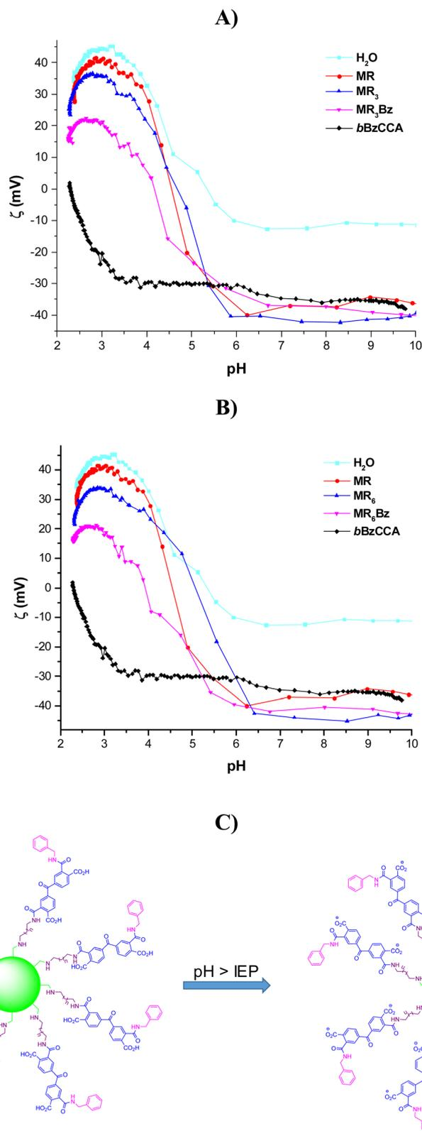
Fig. 6  $\zeta = f[\text{pH}]$  profiles for (A) MR, MR<sub>3</sub> and MR<sub>3</sub>Bz and (B) MR, MR<sub>6</sub> and MR<sub>6</sub>Bz. (C) Schematic of the deprotonation of bCCA molecules attached to the resins, forming negative charges. Mass of resin: 20 mg. Volume: 20 mL. Solvent: deionized water.
