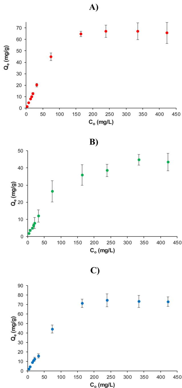
Fig. 9 Non-linear adsorption isotherms of  $\text{Pb}^{2+}$  in (A)  $\text{MR}_3\text{Bz}$ , (B)  $\text{MR}_4\text{Bz}$  and (C)  $\text{MR}_6\text{Bz}$  resins. Mass of resin: 10 mg. Volume: 10 mL. Solvent: water. pH: 5.0.
