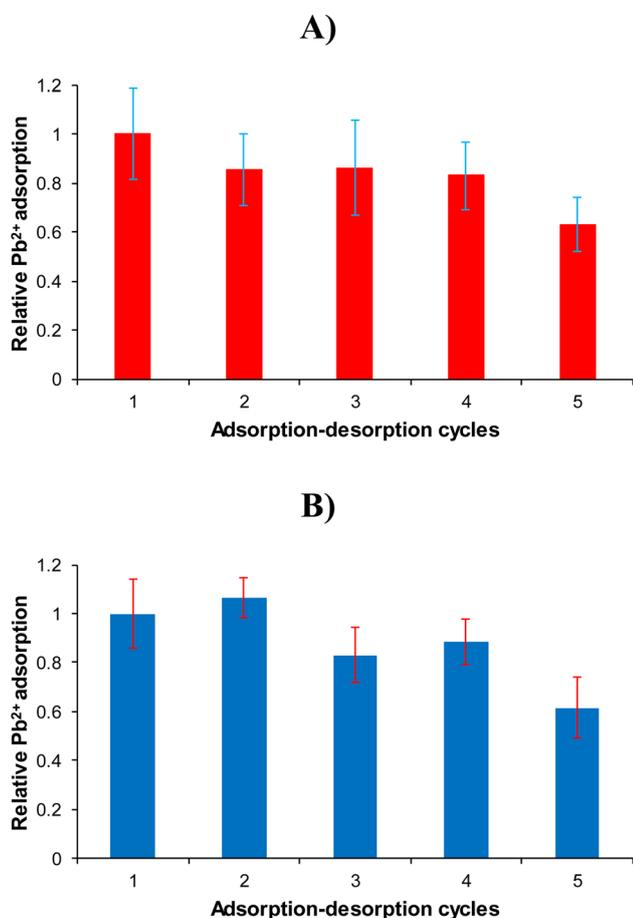
Fig. 10 Relative  $\text{Pb}^{2+}$  adsorption in several adsorption–desorption cycles for (A)  $\text{MR}_3\text{Bz}$  and (B)  $\text{MR}_6\text{Bz}$  resins. Mass of resin: 10 mg. Volume: 10 mL. Solvent: water. pH: 5.0.
