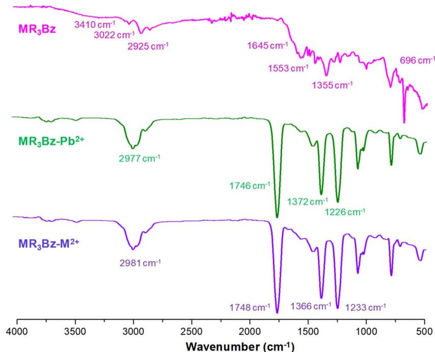
Fig. 12 FTIR spectra of pristine MR<sub>3</sub>Bz (magenta), Pb<sup>2+</sup>-loaded MR<sub>3</sub>Bz (green) and M<sup>2+</sup>-loaded MR<sub>3</sub>Bz (purple) resins obtained under a N<sub>2</sub> atmosphere. M<sup>2+</sup> denotes a mixture of divalent cations.
