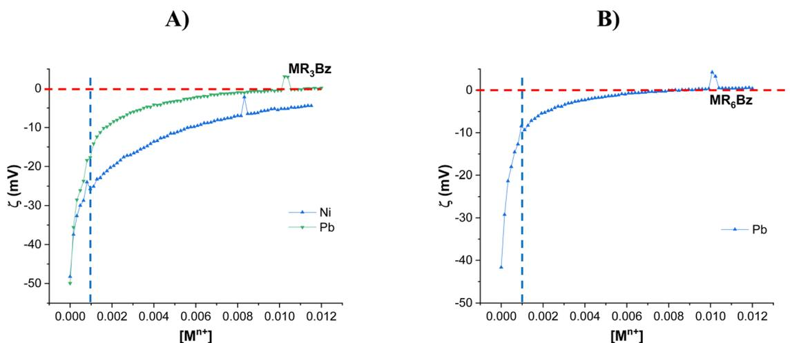
Fig. 7  $\zeta = f[M^{n+}]$  profiles of MR<sub>3</sub>Bz (A) and MR<sub>6</sub>Bz (B) with different metal ions. Mass of resin: 20 mg. Volume: 20 mL. Solvent: deionized water. pH: 5.0.
