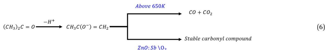
It is important to notice that acetone treatment did not lead to any significant enhancement in the resistance, as shown in Fig. 4 above. Therefore, the acetone path of the reaction (*i.e.* the dehydrogenation shown in eqn (5) and (6)) is quite unlikely to be the responsible mechanism for the observed resistance enhancement. This leaves us with one likely reaction path, which is the propylene-producing dehydration path outlined in eqn (7) below.
