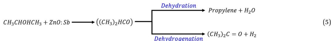
In the dehydrogenation path, an enolate anion is formed by the abstraction of a proton from one of the methyl groups of acetone. This enolate intermediate oxidizes by an ambient oxygen molecule on the ZnO:Sb surface, thus speeding the process of oxygen adsorption to the surface.<sup>29,31</sup>
