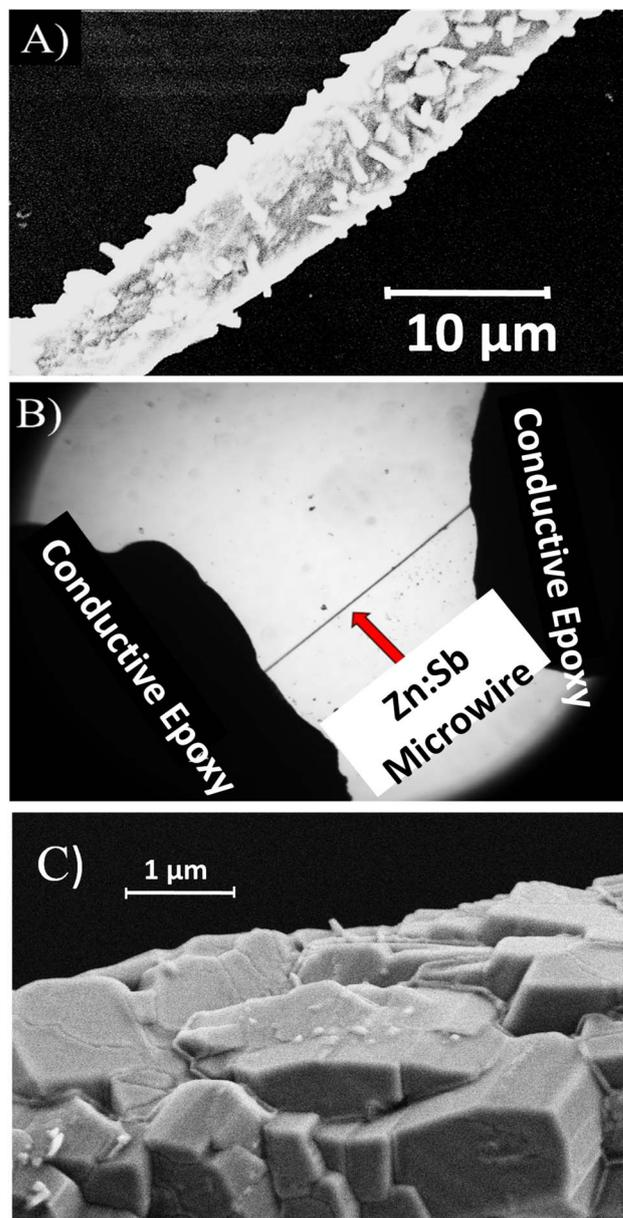
Fig. 1 (A) SEM image for ZnO:Sb micro-wire. The surface of the wire is not smooth and has many nano-crystals on it (B) optical microscope image of a ZnO:Sb micro-wire that has been connected to the measurement circuit using two conductive epoxy drops. (C) High-resolution SEM image showing the rough, polycrystalline nature of the ZnO:Sb wires surface.
