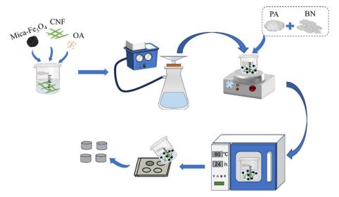
Fig. 1 Schematic of the preparation procedure for mica-Fe<sub>3</sub>O<sub>4</sub>/CNF/BN/PA.
