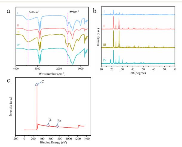
Fig. 2 FT-IR, (a) XRD, (b) and XPS (c) analysis of CPCMs (I: mica/PA, II: mica/BN/PA, III: mica/CNF/BN/PA, IV: mica-Fe<sub>3</sub>O<sub>4</sub>/CNF/BN/PA).
