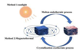
Fig. 8 Schematic of photothermal conversion and magnetothermal conversion.
