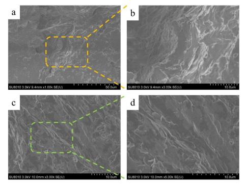
Fig. 3 Top views (a and b) and cross-sectional images (c and d) of CPCMs.
