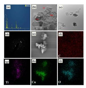
Fig. 2 (a) EDS spectrum, (b-d) TEM images, and (e-i) elemental mapping images of TCC 8 NCs representing elemental C, Ti, Cu, and O.
