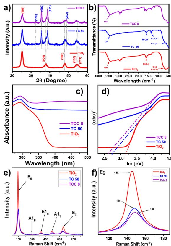
Fig. 1 (a) XRD patterns, (b) FT-IR spectra, (c) UV-visible DRS, (d) Tauc plots, (e) Raman spectra, and (f) localized magnified Raman spectra of bare TiO<sub>2</sub> NPs, TC 50 NCs with varying content of CuO (50 wt%), and TCC 8 NCs with varying content of CS NPs (8 wt%).
