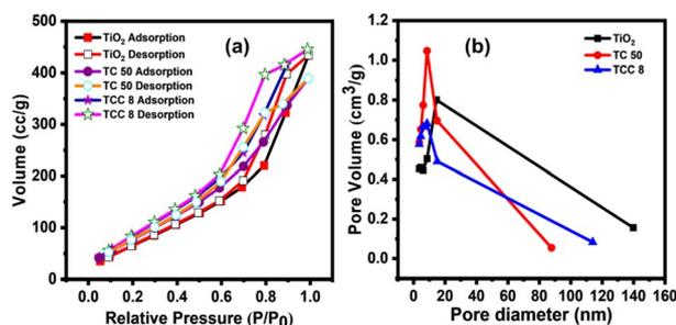
Fig. 3 (a) N<sub>2</sub> adsorption–desorption isotherms, and (b) BJH curves of bare TiO<sub>2</sub> NPs, TC 50 and TCC 8 NCs.
