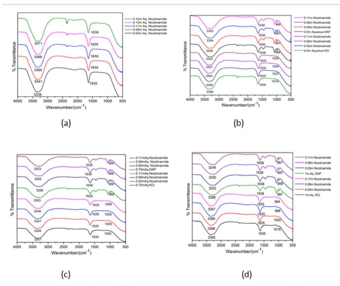
Fig. 4 FTIR spectra of (a) aqueous NA (NA +  $H_2O$ ) (b) 0.05 m, 0.09 m, 0.11 m NA with 0.5 m DAP and 0.5 m KCl respectively. (c) 0.05 m, 0.09 m, 0.11 m NA with 0.75 m DAP and 0.75 m KCl respectively. (d) 0.05 m, 0.09 m, 0.11 m NA with 1 m DAP and 1 m KCl respectively.
